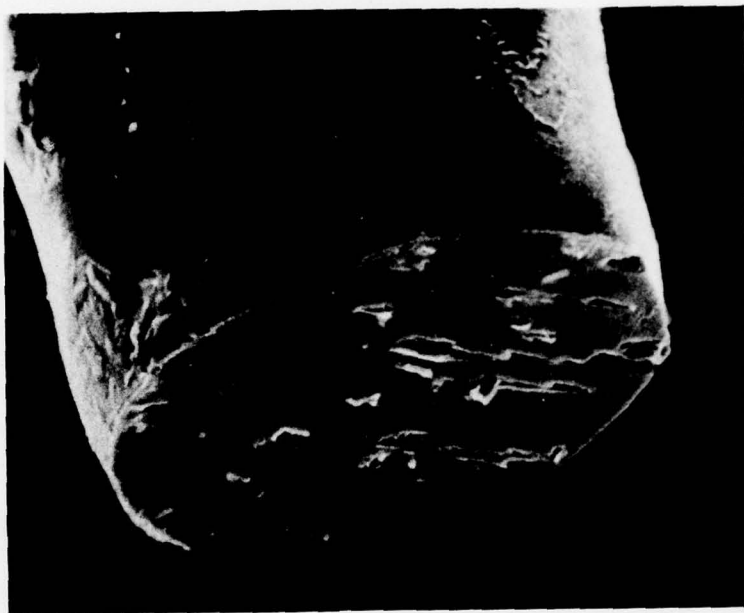
Figure 3 - Fracture of vanadium specimen annealed at 1700° C for 25 hours (S.E.M. 700X)
