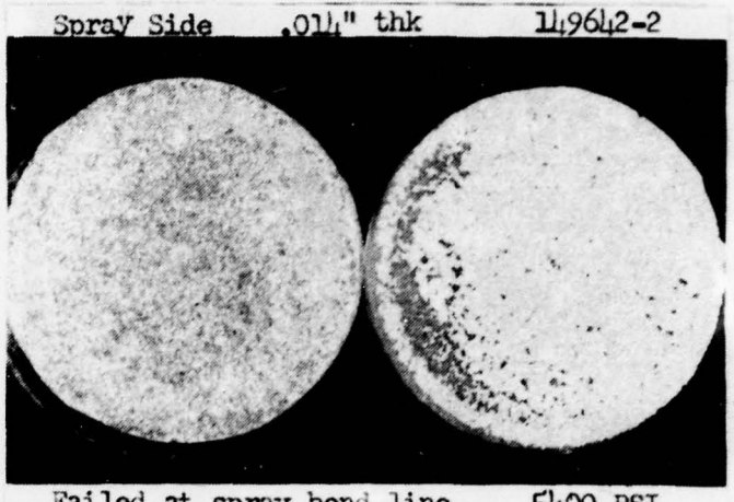
Failed at spray bond line 5400 PSI
