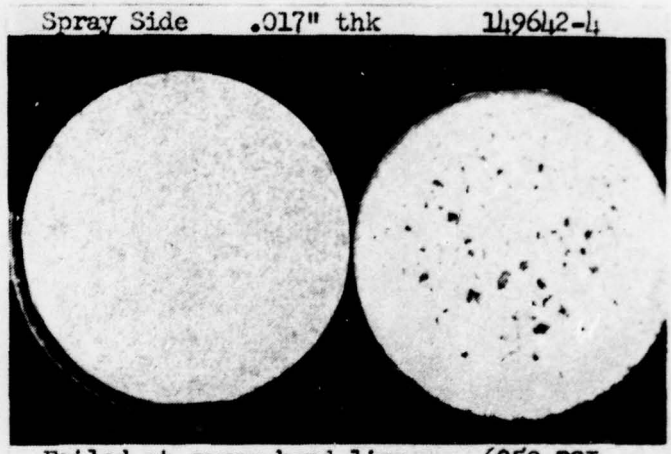
Failed at spray bond line 6250 PSI
