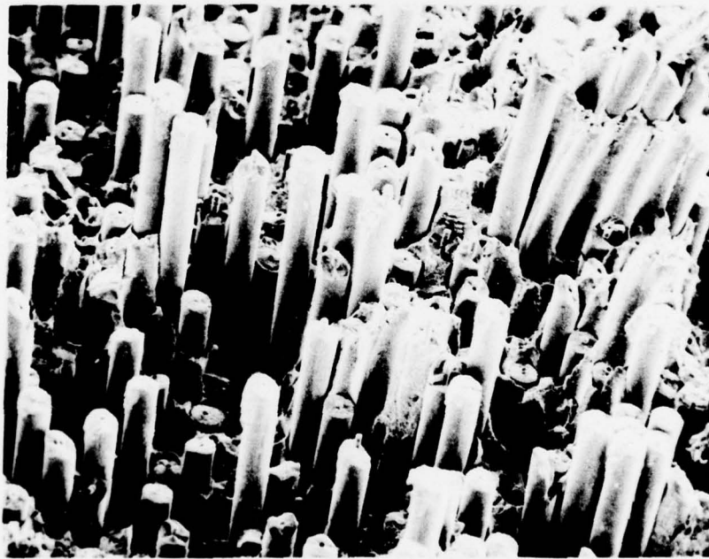
FIG. 21 FRACTURE SURFACE OF CHARPY IMPACT SPECIMEN 50% AVCO SiC REINFORCED 6061
