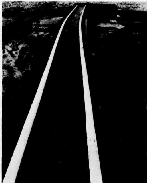
Photo A14. Looking downstream at flow slot with diversion gate open, Q = 5,000 cfs
