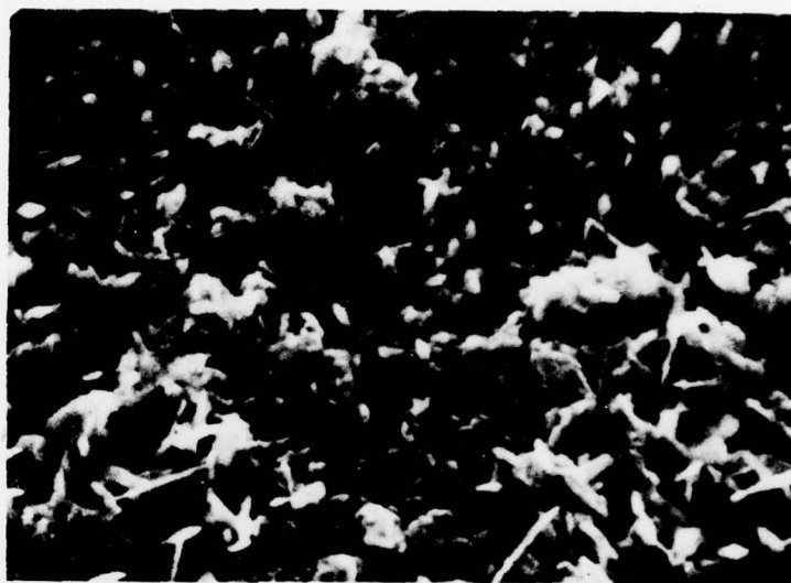
Fig 16 Alloy heat treated at 740°C for 3 hours.
