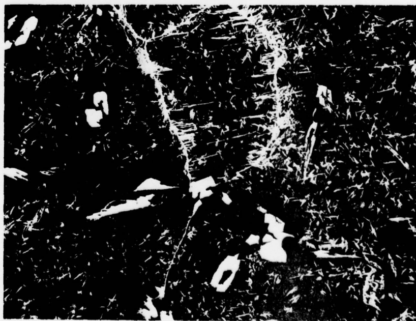
Fig 5 Alloy slowly cooled from 1000°C to 900°C and quenched, showing nucleation of \alpha phase.
