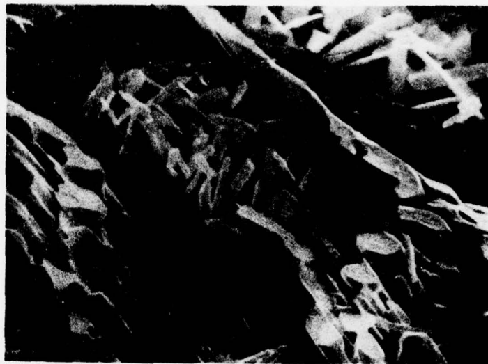
Fig 18 Alloy heat treated at 840°C for 3 hours.
