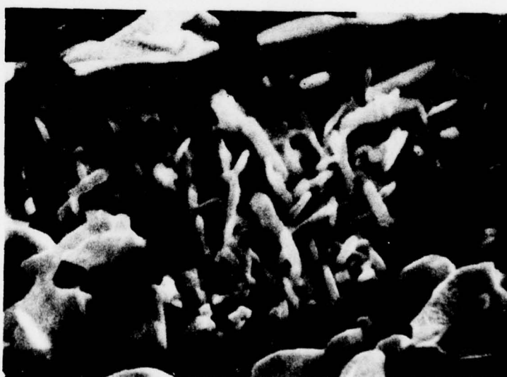
Fig 17 Alloy heat treated at 790°C for 3 hours.
