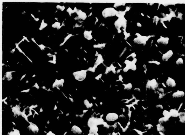
Fig 19 Alloy heat treated at 675°C for 6 hours showing lath and globular precipitates.
