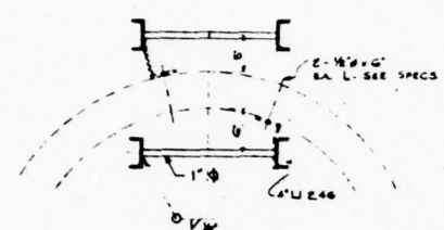
SECTION 1-1 TYPICAL AT 48" PIPE BAZZEL
