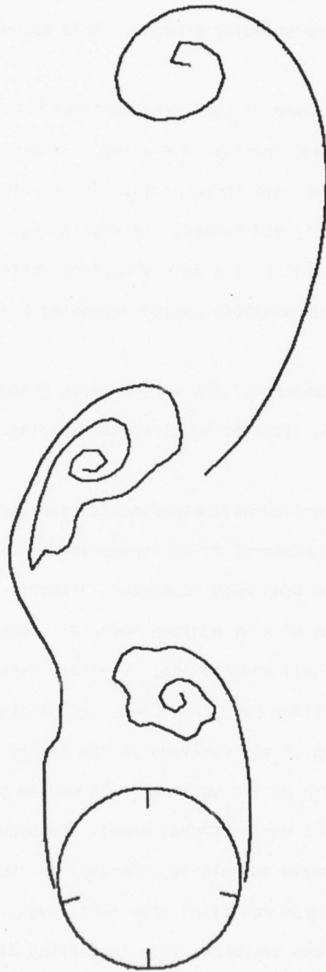
Fig. 14 Initiation of vortex-shedding sequence
