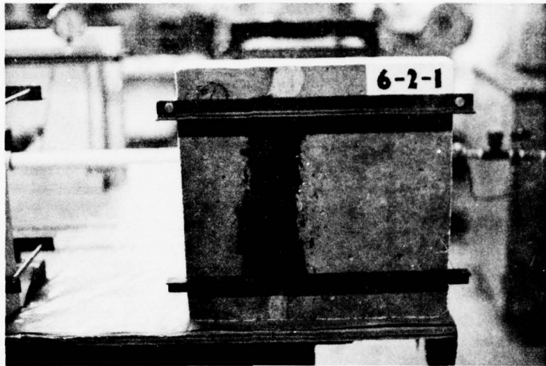
Figure 15. Specimen 2 -- Tremco 50V, no primer (tar/urethane, 2-comp).
