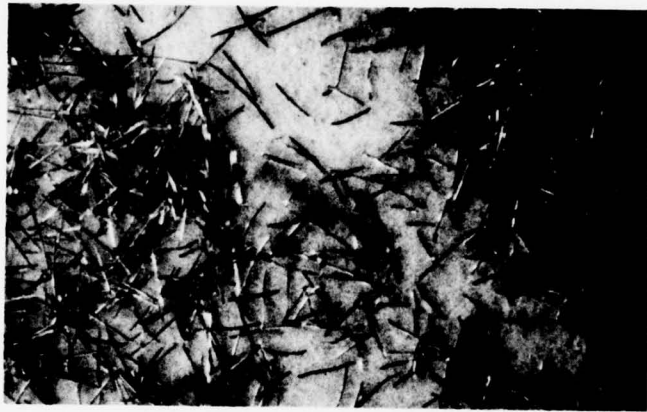
Figure 1 - 0.001-Inch Diameter Chopped Copper Wire, 0.032/0.042 Inch Long (Photomicrograph of Unblended Chopped Wire (15X))
