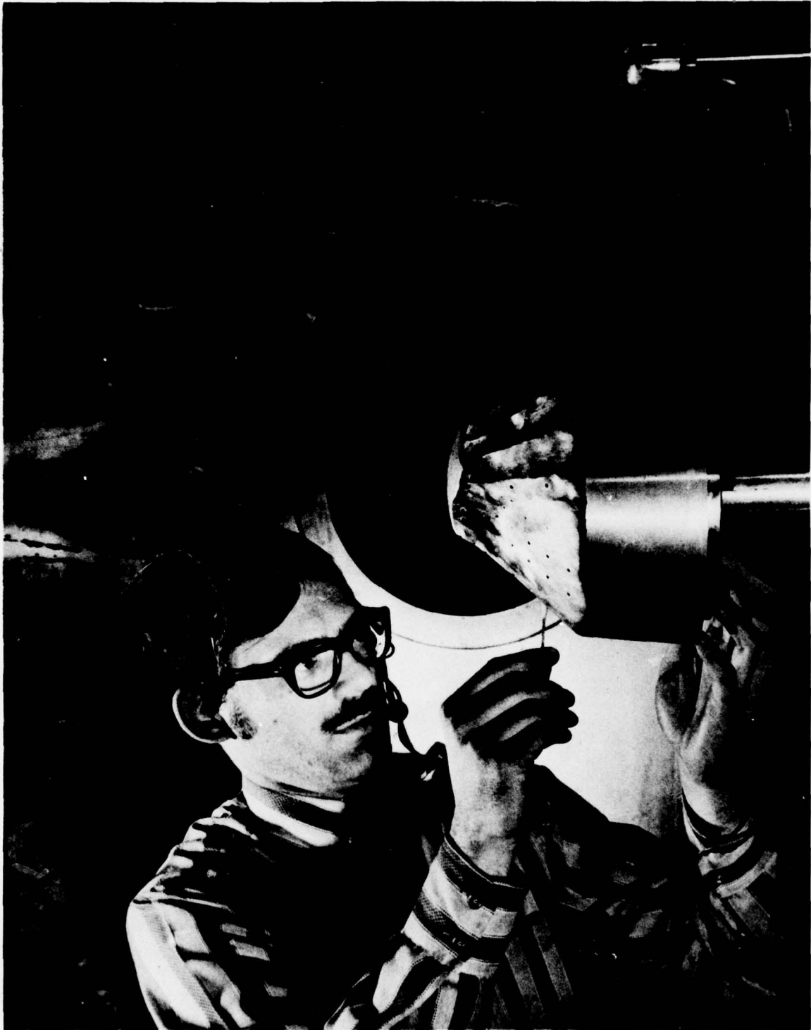
Figure 5-3a INSTALLATION OF NRV HEAT TRANSFER AND PRESSURE MODEL IN 96" SHOCK TUNNEL
