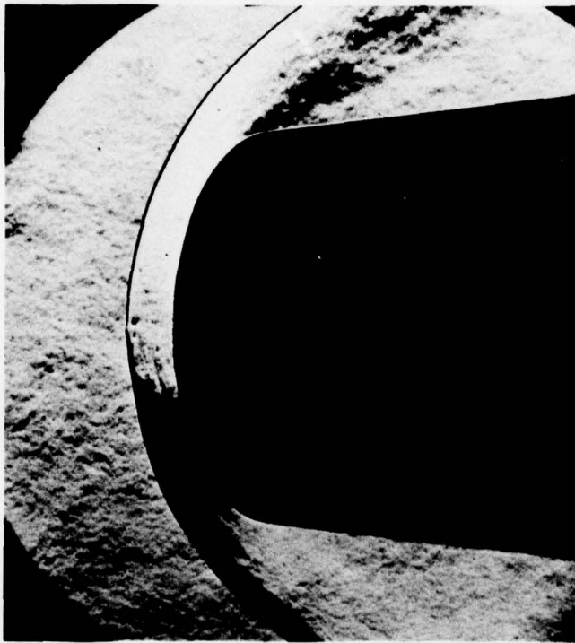
Figure 6-1a SHOCK-PARTICLE INTERACTION OVER A BLUNT ELLIPSOID
