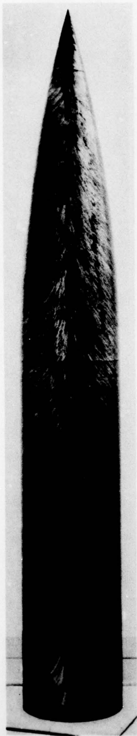
Figure 19.- Carbon black surface flow visualization, \alpha = 22\text{-}1/2^\circ ; Re_D = 0.37 \cdot 10^6 .
