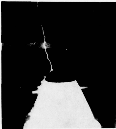
Figure 7b. 0° Lightning Strike to Diverter Strip #2.
