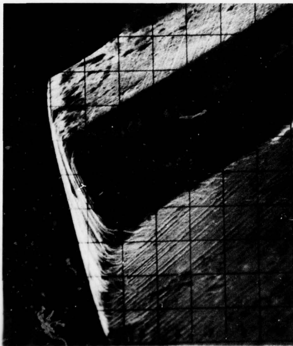
Figure B28. Micro Grade Drill - 140° Point, 20° Relief - After 4200 Hits
