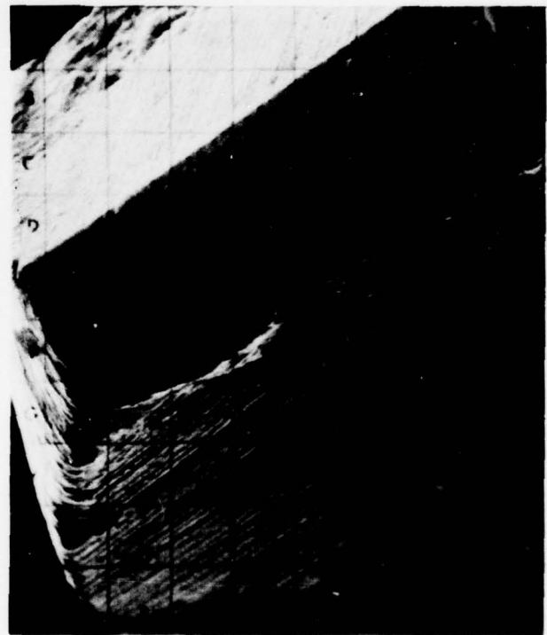
Figure B8. Fine Grade Carbide Drill w/Microlube - After 4200 Hits
