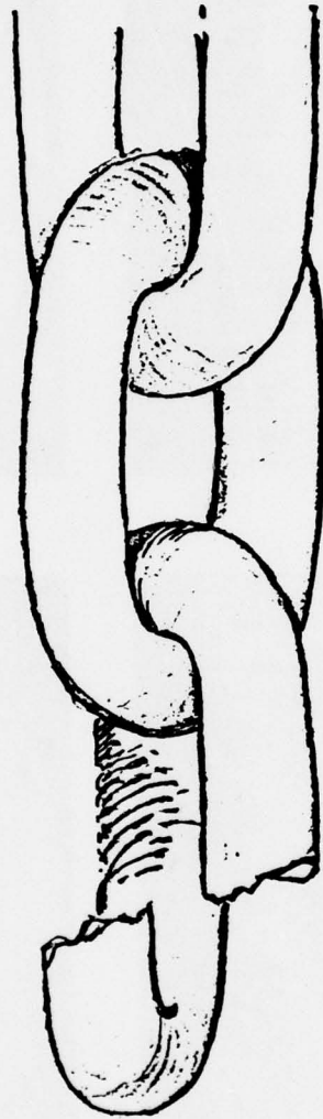
Figure 1. Isometric representation of NIKE-HERCULES hoisting chain as received.
