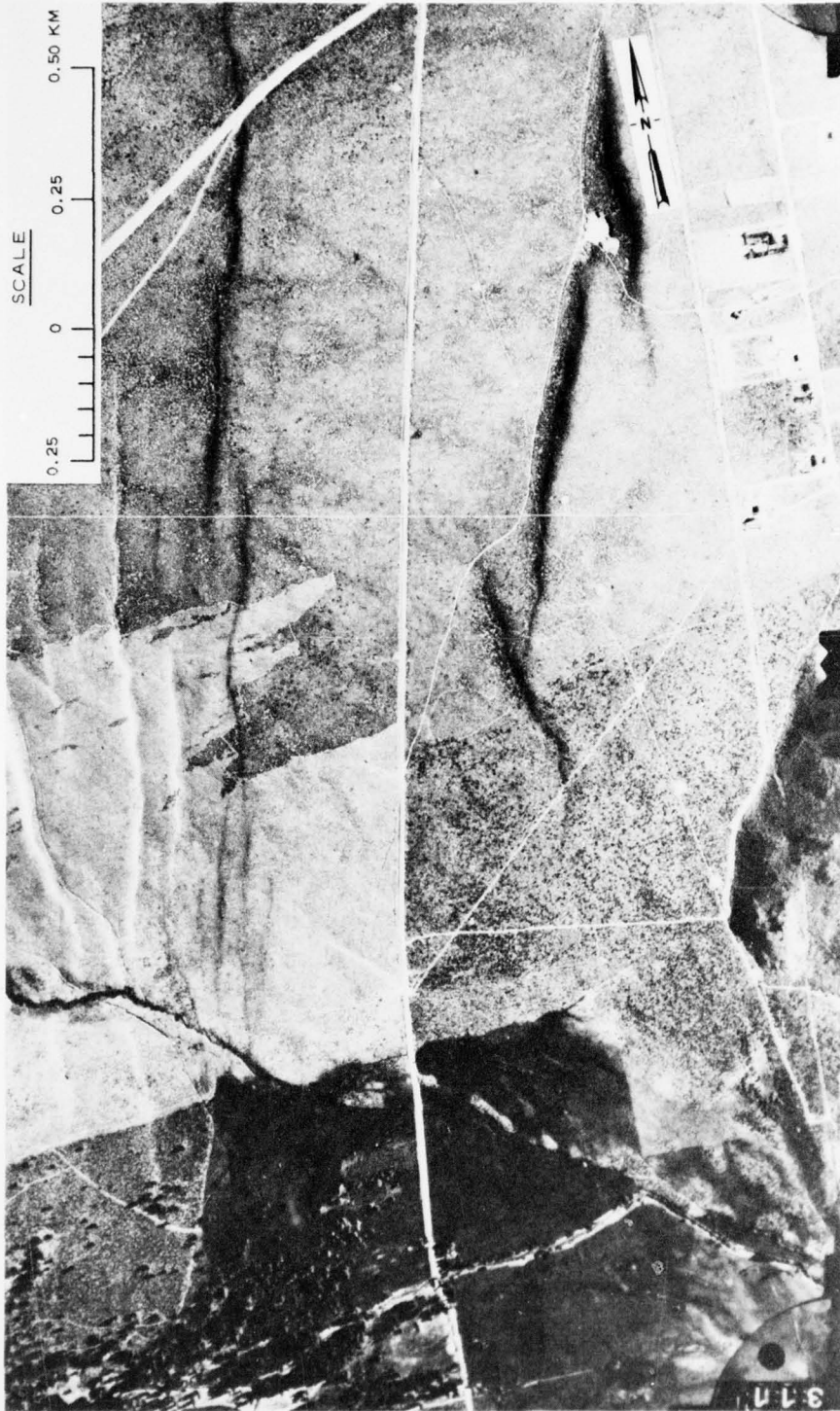
Figure 38. Vertical aerial photograph showing fault swarm in Quaternary alluvium, about 10 miles south of Reno, Nevada. The photograph is taken with a sun angle azimuth of N77^{\circ}E and 25^{\circ} inclination. Scarps steeper than 25^{\circ} cast deep shadows, if west-facing, and have bright highlighting where east-facing. More gentle west-facing slopes have lighter grays on less bright highlighting, respectively
