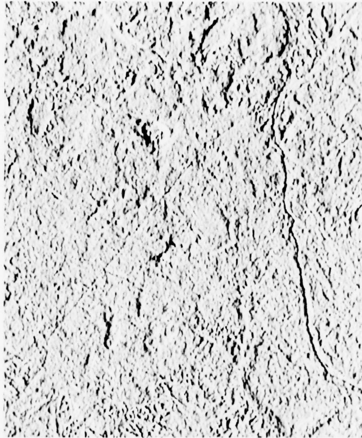
Figure 111. High-pass filter of a band 5/band 6 ratio. This scene near Flagstaff, Arizona, displays numerous northwest-southeast lineaments which are not apparent on the original band 5 and band 6 images. The diagonal feature extending from the lower left to the upper right is a highway. (Image processed by Dr. Robert A. Schowengerdt, Assistant Professor of Remote Sensing, University of Arizona)
