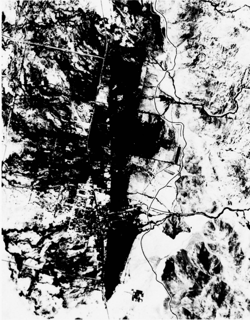
Figure 8. Vertical aerial photograph of Owens Valley, California. The Owens Valley fault extending nearly horizontally across the photograph causes a vegetation contrast through the town of Lone Pine, California. Though the fault scarp, which broke in 1872, has been modified by agriculture activity, it is discernable on aerial photography due to the vegetation contrast
