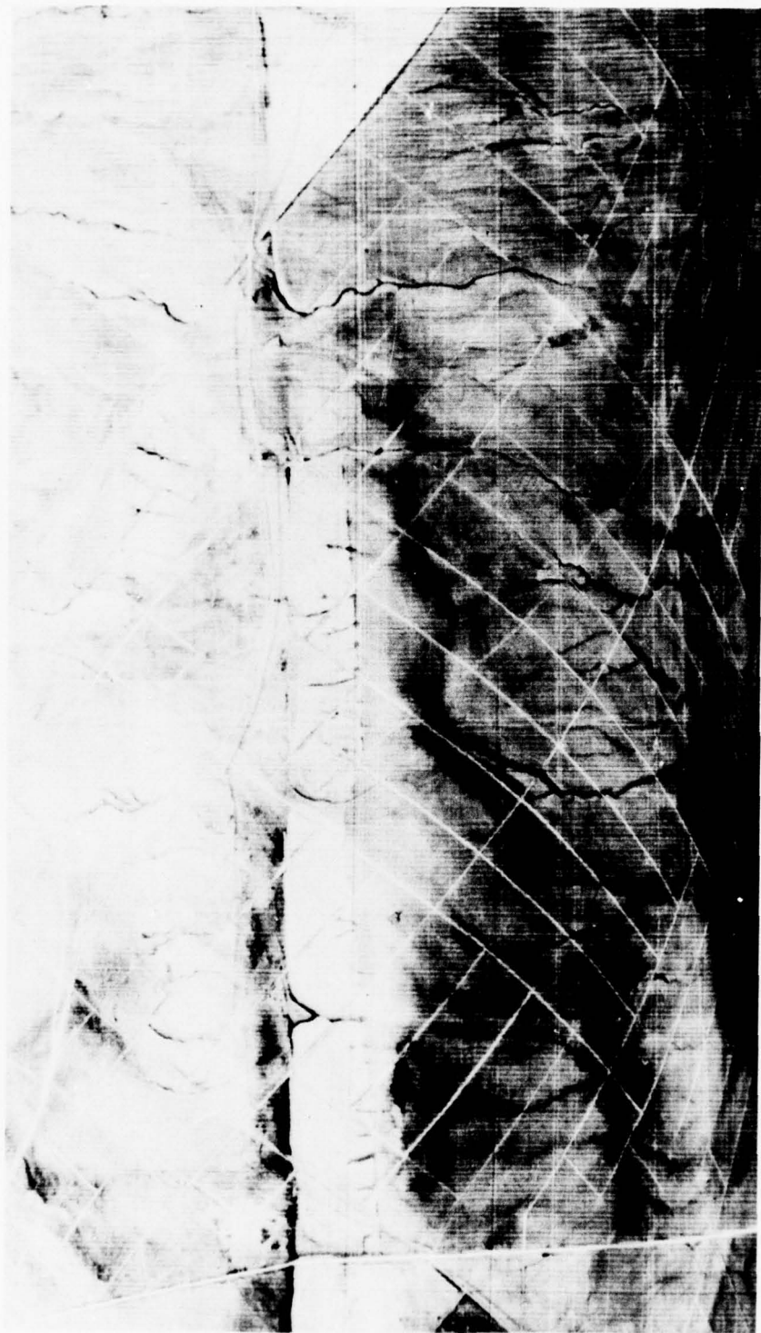
Figure 79. Thermal infrared image of the San Andreas fault, California. This image of the same area as Figure 78 shows the main scarp of the San Andreas fault as a sharp contrast in tone. The darker areas correspond to cooler areas, and the tone contrast is due to near-surface moisture on the east side of the fault and a relatively warmer ridge on the west. The subparallel branches (Figure 78) are not visible on the thermal scan and the orthogonal road system has been transformed into a curvilinear system due to the scanner. Significant geometrical corrections and field checks are required before accurate mapping may proceed
