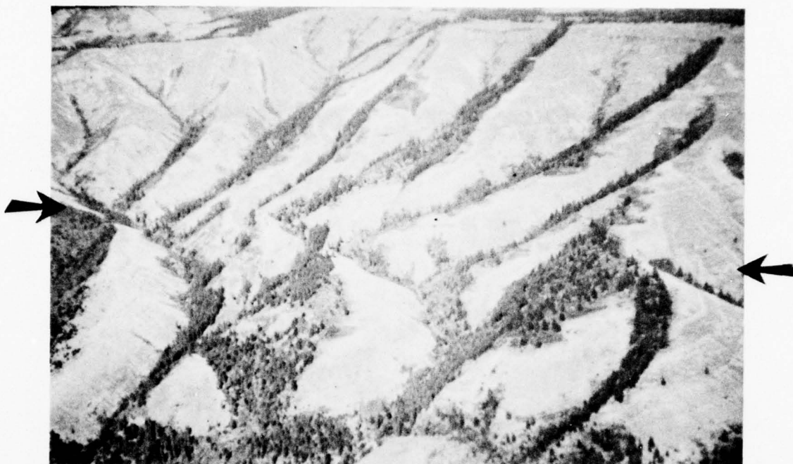
Figure 34. Low oblique photograph of fault near Walla Walla, Washington. Disruption and funneling of the streams are caused by a fault which extends from left to right across the center of the photograph. Though there is no scarp, the fault can be traced on imagery for several kilometres because of its effect on drainages
