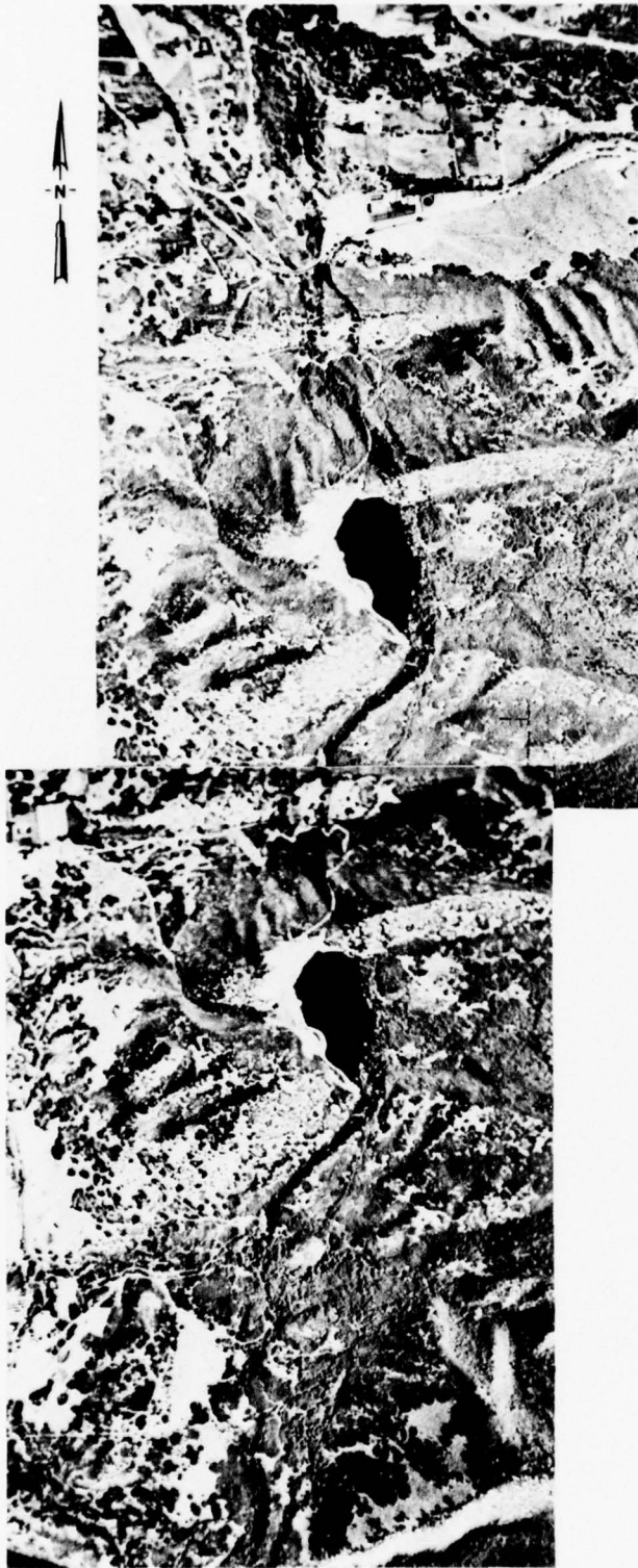
Figure 18. Stereopair photographs of Bells Canyon, Utah. The active Wasatch fault can be seen displacing the moraine at the mouth of Bells Canyon. The scarp is over 30 m high across the moraine, and although the scarp is accentuated by low-angle sunlight, the main fault scarp and some secondary scarps can be mapped using parallax, whereas in a single photograph they are not as apparent
