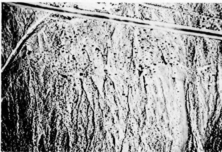
Figure 31. Vertical aerial photograph of Owens Valley, California. The graben located just below the road (arrow) can be delineated by the incised stream erosion on the upthrown sides. The irradiation direction is parallel to the scarps but perpendicular to the streams making the change in erosion characteristics stand out
