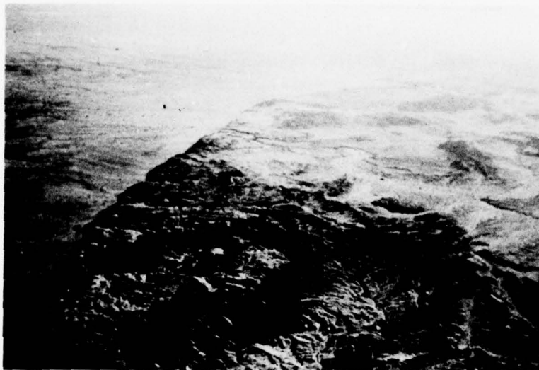
Figure 5. San Andreas Fault, Imperial Valley, California. The San Andreas fault is dramatically marked in this high oblique photograph by the change in texture across the fault. The stream patterns and fracture patterns in the foreground are more dense and deeply incised than the patterns across the fault. Note the fault at the lower center of the photograph which brings a light-toned rock into juxtaposition with the dark-toned, deeply incised rock
