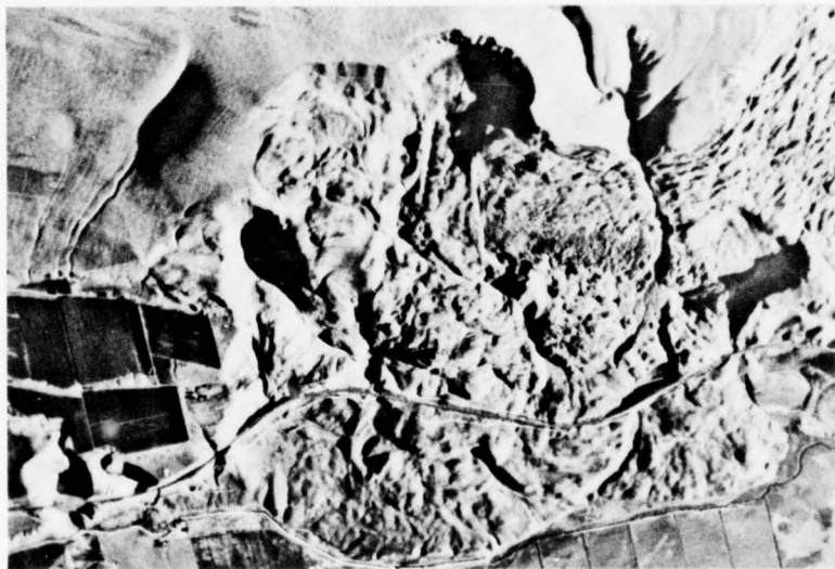
Figure 51. Vertical aerial photograph of a large landslide near Corfu, Washington. The disrupted surface topography of the slide debris is characteristic of a relatively fluid slide mass. Note the hummocky texture of the slide mass in the lobate edges at the lower portion of the photograph
