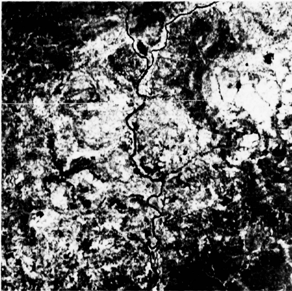
Figure 102. Logarithmic contrast stretch of Figure 101. Darker tones have been stretched more relative to lighter tones. Thus, the darker areas show more contrast and the lighter areas show less contrast than Figure 98a and b
