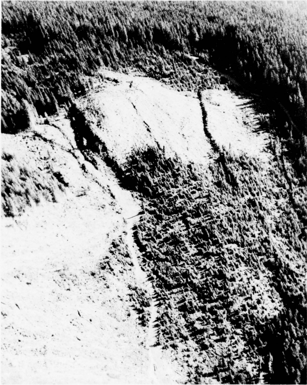
Figure 124. Straight Creek fault zone on Diobsud Ridge, Bacon Creek area. The scarp in the clearcut is viewed from the south. There are two postglacial, back-facing or antislope scarps on the clearcut
