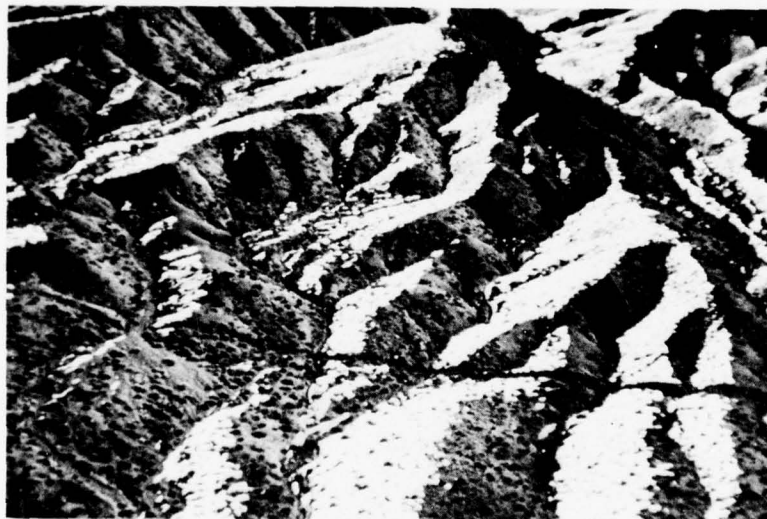
Figure 29. Low oblique view of 1954 Gold King fault on eastern edge of Dixie Valley, Nevada. The lack of snow on the south side of small ridges and the shading effect combine to make the scarp especially conspicuous and enhance the right-slip offset of the ridge crests and ravines on the right side of the photograph
