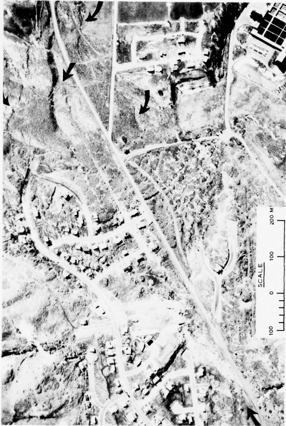
Figure 117. Vertical photograph of Wasatch fault, Utah, taken in 1969. It shows several recent scarps (arrows) of the Wasatch fault north of Little Cottonwood Canyon (dotted on Figure 116). The shatter zone extends to beyond the water filtration plant (lower right corner). The fresh nature of the scarps, the sharp "y" shaped canyons, active fan deposition, and lack of sinuosity of the Wasatch range front indicate a tectonically very active area. Development along and within the fault zone is exemplified by the new subdivision
