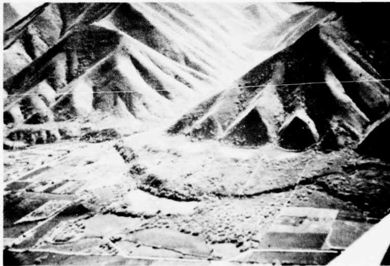
Figure 44. Low oblique photograph of the Wasatch fault near Springville, Utah. A closer view than Figure 39, this photograph exemplifies the irregular character of the most recent fault scarp
