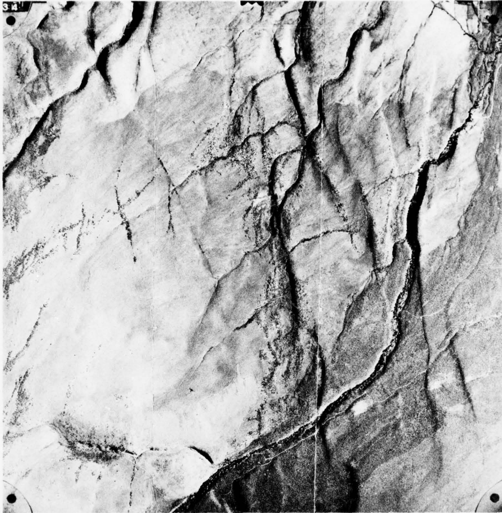
Figure 12. Vertical aerial photograph showing complex swarm of branching fault scarps near Reno, Nevada. The northerly trending scarps are generally marked by alignments and clusters of larger shrubs. The low morning sunlight from N78^{\circ}E (right of photograph) highlights the east-facing scarps and shades the steeper parts of the west-facing scarps. The angle of sun incidence is at an inclination of 23^{\circ} . The steeper west-facing scarps are in full shadow and the more gentle older, and more deeply weathered scarps with slopes from 5^{\circ} to 23^{\circ} have various lighter gray tones, with the tone related to scarp angle
