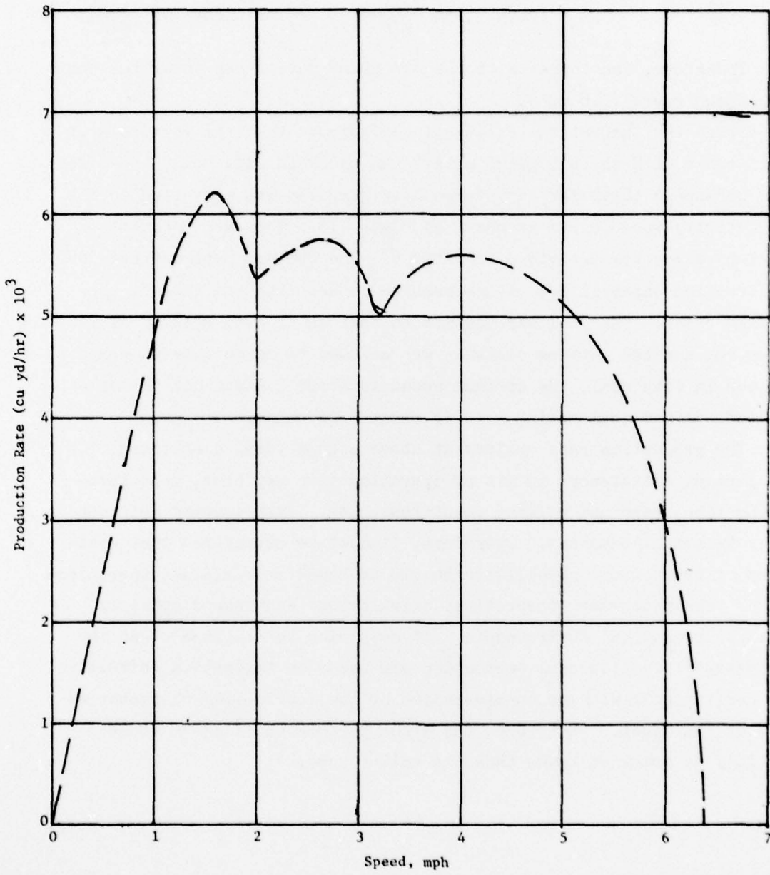
Figure 15. Estimated production rate versus speed for the Holland loader, Series H1 with 41B prime movers on in situ coal
