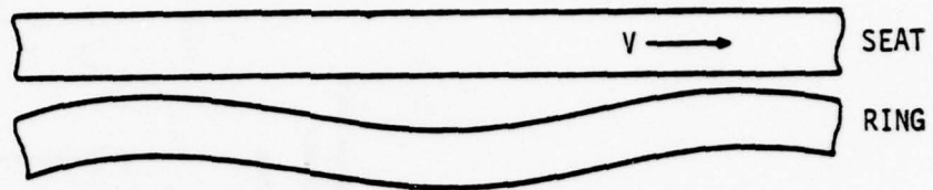
DISTORTED RING UNDER ZERO PRESSURE
