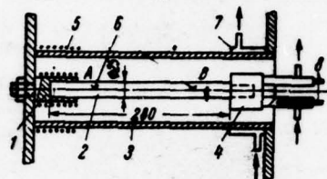
Fig. 4.1. Diagram of installation of Williams [4-4]. 1 - block/module/unit of heater; 2 - specimen/sample; 3 - guard cylinder; 4 and 7 - coolers; 5 - heater of guard cylinder; 6 and 8 - thermocouple.
