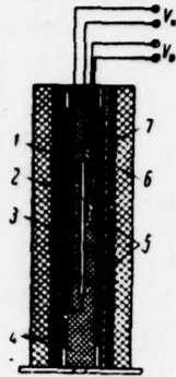
Fig. 4.2. Diagram of installation of Hagan and Sawyer [4.11]. 1 - heater - source of heat flux; 2 - specimen/sample; 3 - leveling cylinder; 4 - insulation/isclation; 5 - thermocouple; 6 - heater of furnace; 7 - jacket of furnace.
