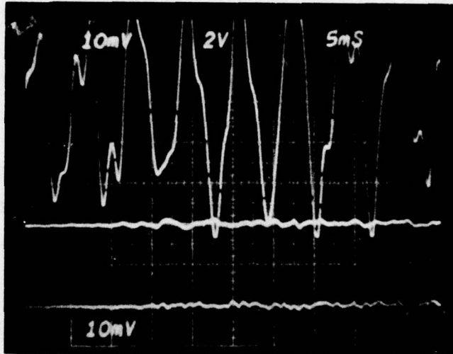
Figure 8n - Change in Forward Voltage Drop During Blow 222
