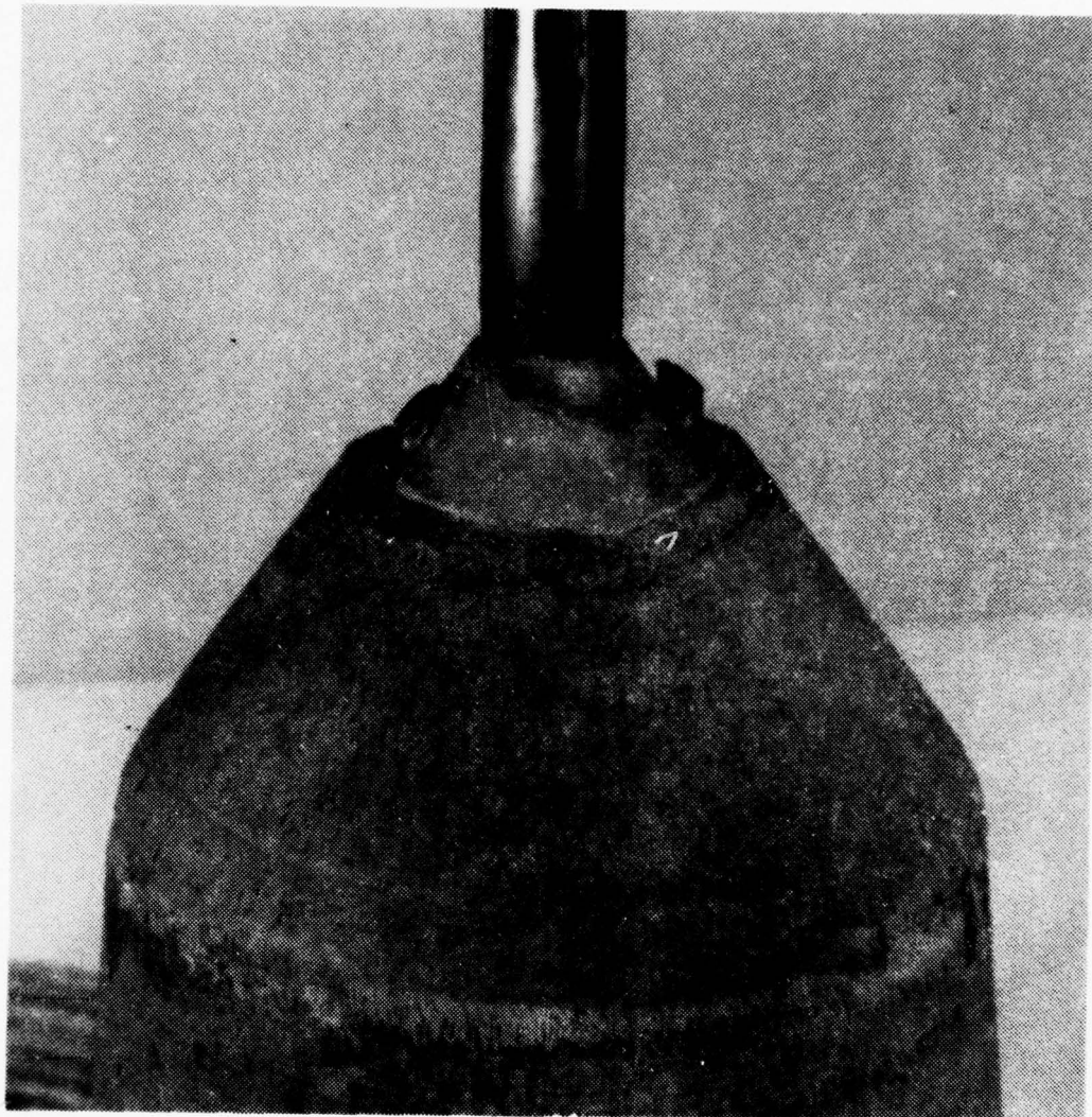
Figure 4-13. Damaged boom and drogue heatshield.
