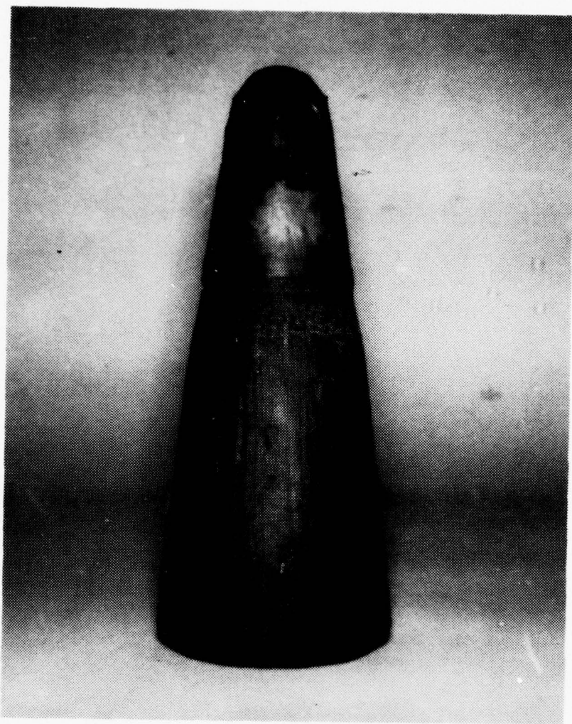
Figure 4-14. Recovered tungsten nosetip from FLAME F-005.
