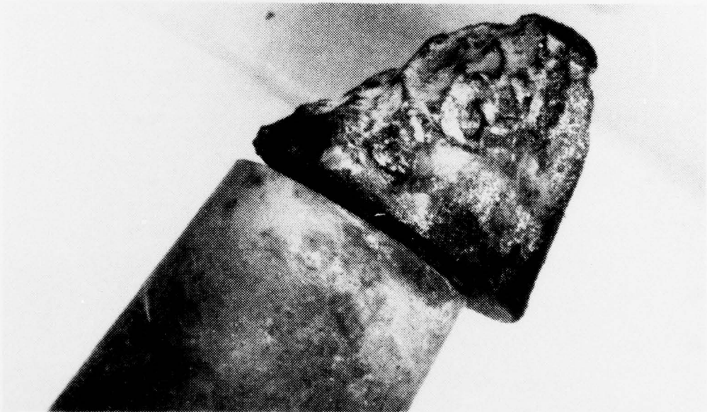
Figure 4-27. Recovered gasjet nosetip from FLAME F-008.
