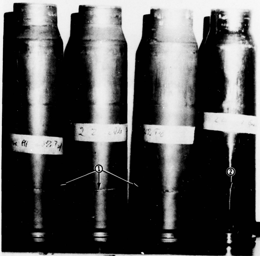
Figure 7. Four cases from Group B showing (1) cracks in cases coated with 30 percent Teflon over zinc plate and (2) stretch in a case coated with Mader lacquer over phosphate
