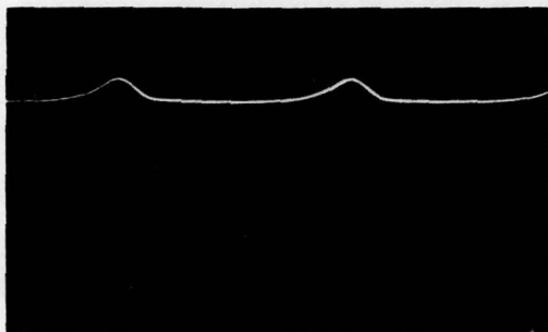
Figure 18. Photographs showing the FACT unit and DACIM I outputs for an input consisting of two sine wave components. The input signal is given by the relation x(t) = A_1 \sin(2\pi f_1 t) + A_2 \sin(2\pi f_2 t) where f_1 = 5010 Hz, f_2 = 5000 Hz, A_1 = 1.1 vrms and A_2 = 1.0 vrms. The FACT unit Doppler scale is approximately 100 Knots/division. The DACIM I Doppler scale is approximately 50 Knots/division.
