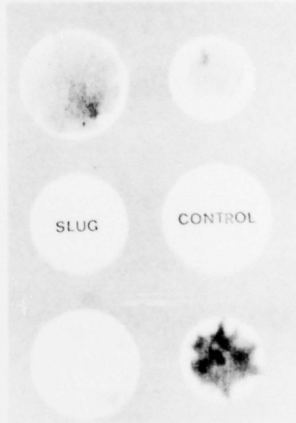
FIGURE 6. Group IV (6.35 mm Air Gap Between Shell Fabric and T-Shirt in Contact With Skin). A. Immediately Postburn; B. 24 Hours Postburn; C. Fabrics: 1-AFN/T/S, 2-Control, 3-NWN/T/S, 4-HT4/T/S, 5-Slug Calorimeter, 6-PBI/T/S; D. FDP on T-Shirt.
