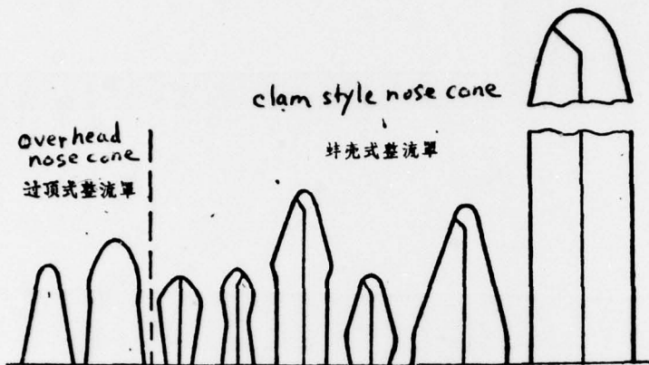
Fig. 2 Several different shapes of nose fairings. Left: overhead fairing; right: clam shell type fairing.
