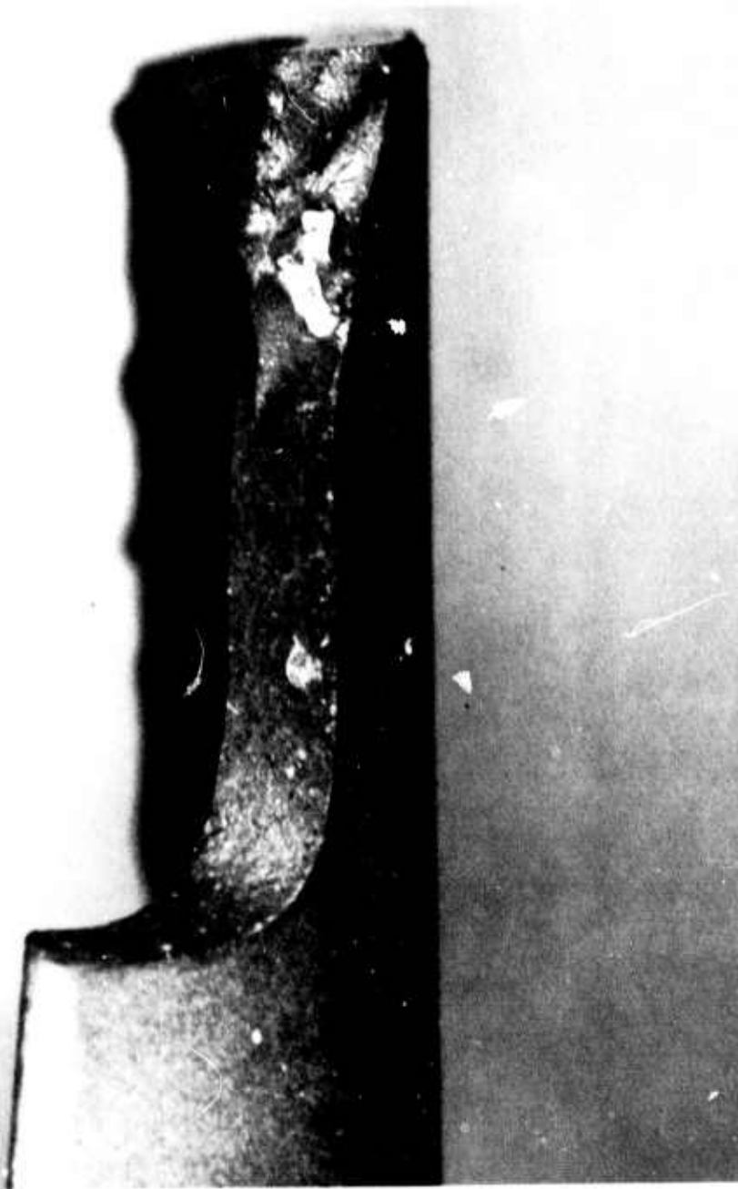
Figure 4.22 Molding Flaw in Reaction Bonded Silicon Nitride Blade — Fractured Surface
