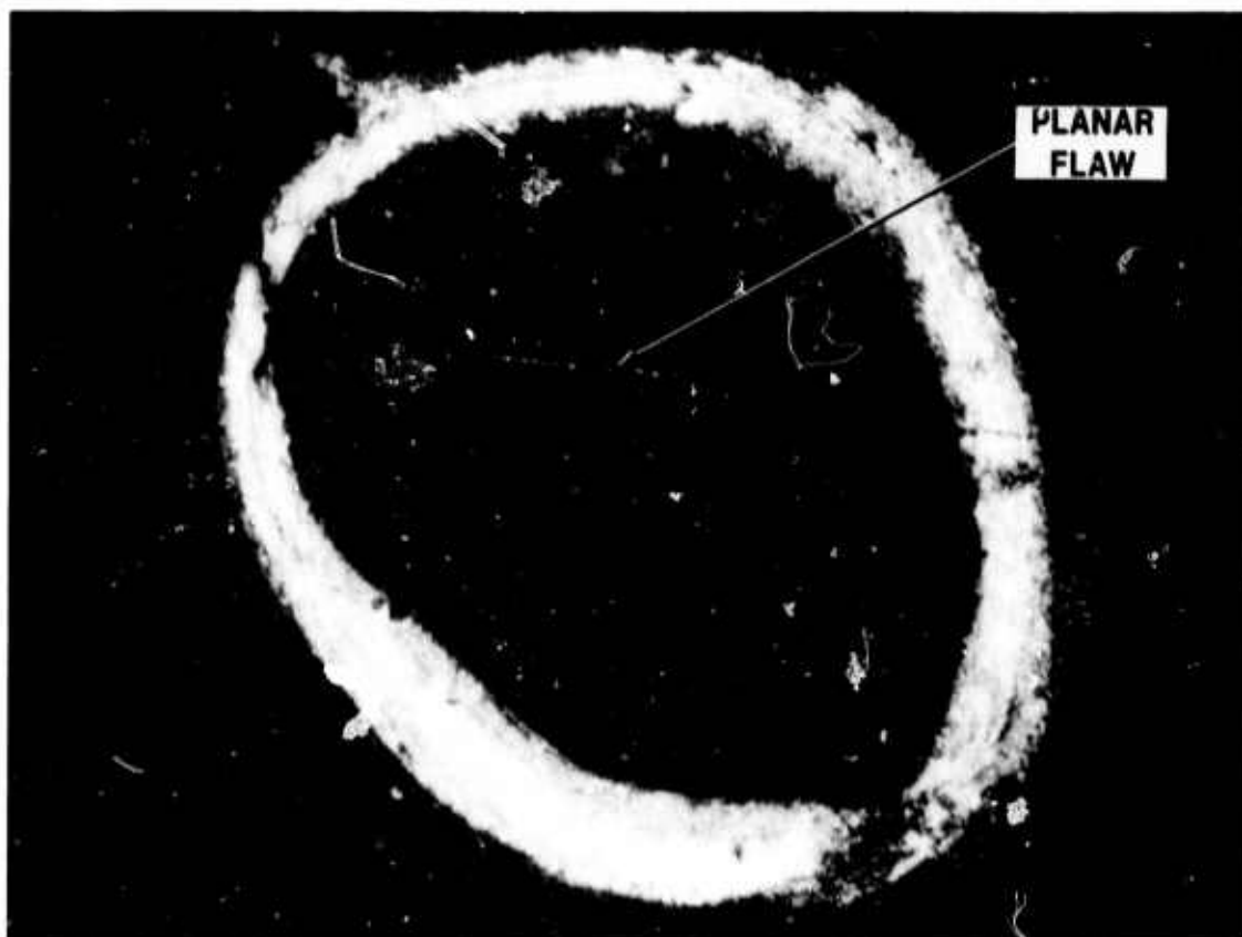
Figure 4.18 Planar Type Defect Detected by Visual Inspection
