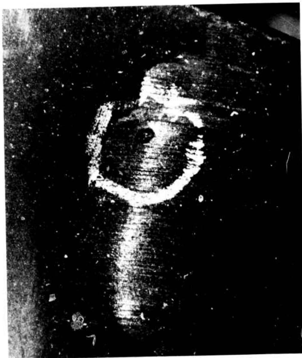
Figure 4.21 Subsurface Void in Reaction Bonded Silicon Nitride Blade Uncovered by Grinding
