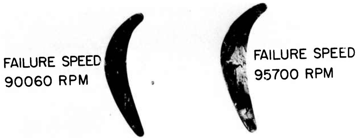
Figure 4.2 Typical Fracture Surfaces without Gross Fabrication Flaws
