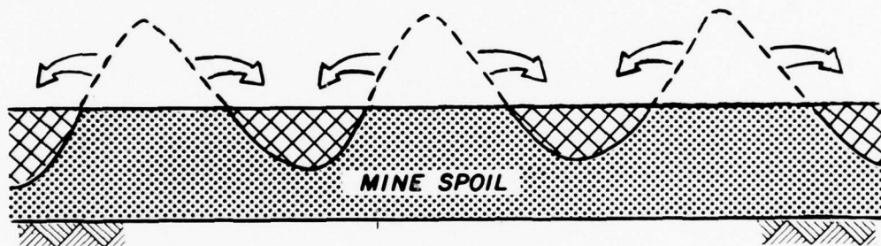
b. Grading the mine spoil
