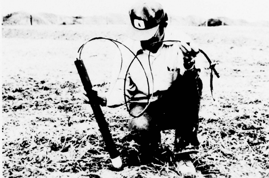
Figure B12. Installing a pressure-vacuum lysimeter for collection of soil water
