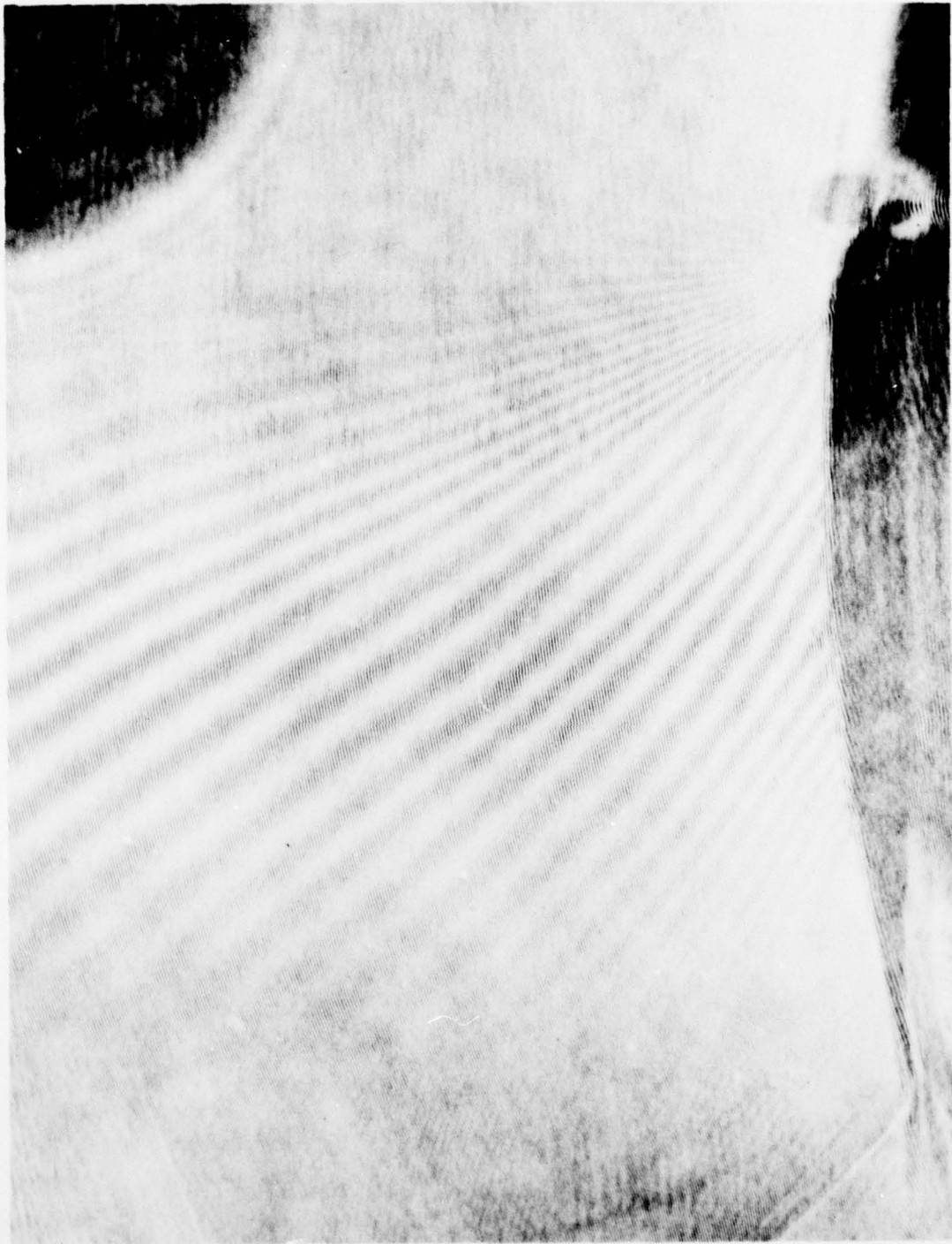
FIG. 14 COMPOSITE INTERFEROGRAM OF UPPER SURFACE FLOW ON SUPERCRITICAL AEROFOIL BGK \approx 1 ( M \approx 1.00 , \alpha = 1.4^\circ , R = 1.2 \times 10^6 )
