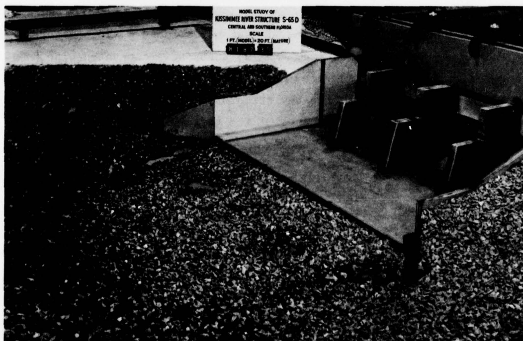
Figure 8. Downstream scour at model structure S-65D, Type 1 design (prototype), after 2-hr test at headwater el 31.24, tailwater el 23.20, all gates open 10 ft
