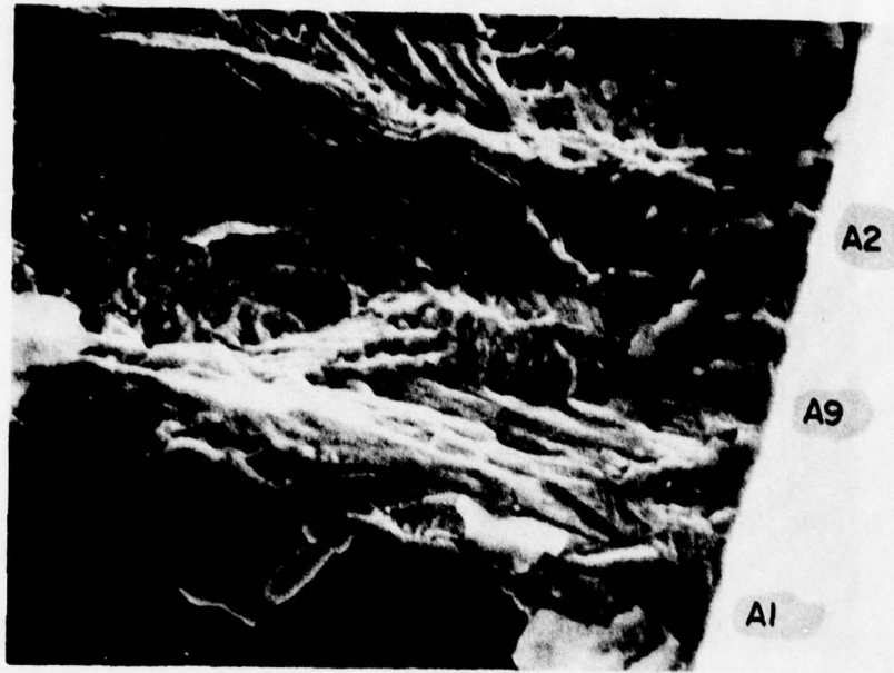
FIGURE 2.28. SPECIMEN NO. 33 VIEWED AT 500 DIAMETERS WITH THE SEM, CRACK INITIATION ZONE
