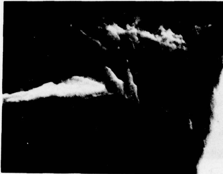
FIGURE 2.29. SPECIMEN NO. 33 VIEWED AT 3000 DIAMETERS WITH THE SEM, CRACK INITIATION ZONE
