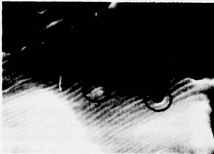
FIGURE 2.33. SPECIMEN NO. 33 VIEWED IN AREA A-8 AT 10,100 DIAMETERS WITH THE SEM SHOWING STRIATION FORMATION AND INTERMETALLIC PARTICLES
