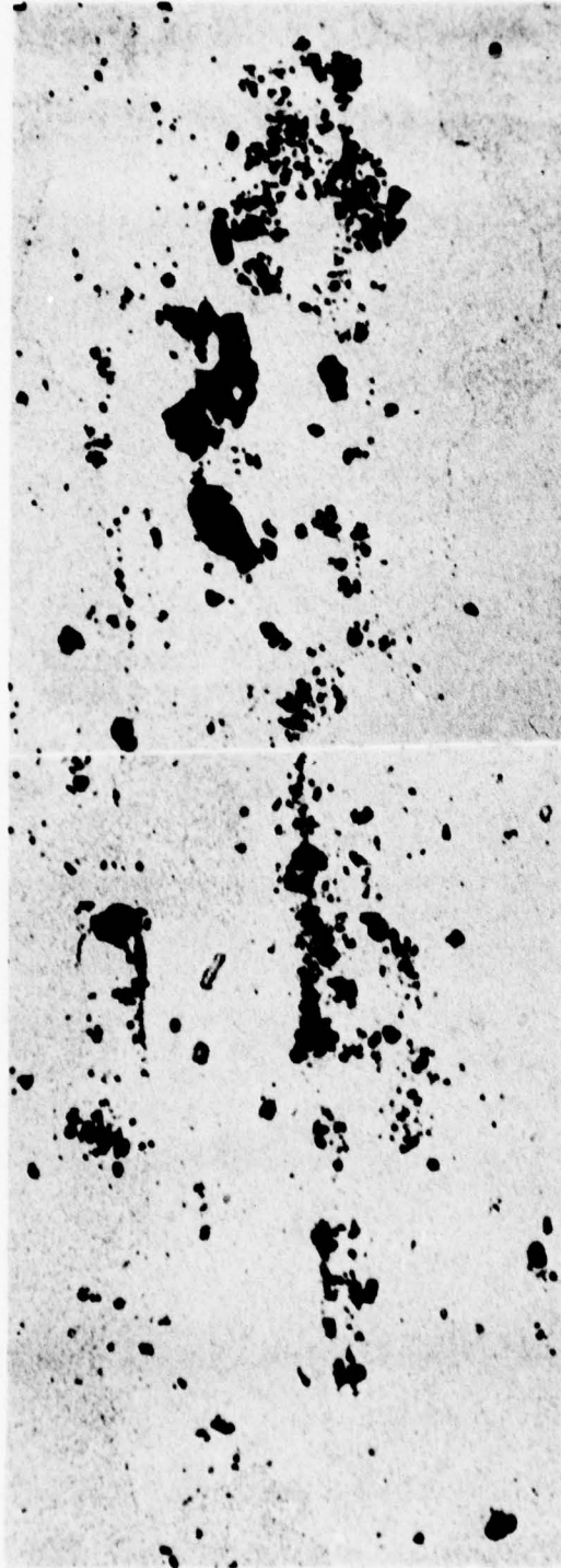
FIGURE 2.12. AN INTERMETALLIC CLUSTER IN PREPARATION B-2, X-Y ORIENTATION VIEWED AT 700 DIAMETERS
