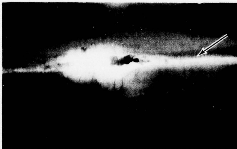
FIGURE 60. PHOTOGRAPH OF X-RAY OF INTERACTION CONDITION ON FLAT AREA ADJACENT TO METAL FLOW CONDITION ON EXTERNAL SURFACE OF PRE-FORM TUBE S/N 6, REFERENCE FIGURE 40. NOTE CRAZING CONDITION IN FLOWED METAL AREA. MAG. 3X.
