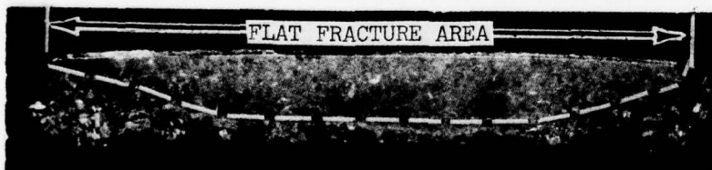
FIGURE 53. FRACTURE INTERFACE OF BEND TEST COUPON S/N 8-2. (START END) NOTE FLAT FRACTURE AREA. MAG. 2X.
