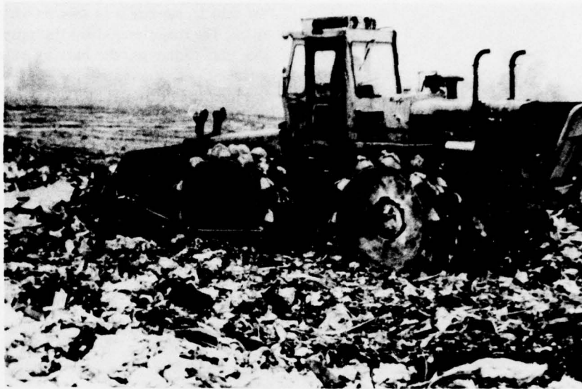
Figure 10. Raygo Rampak 45 compactor.
