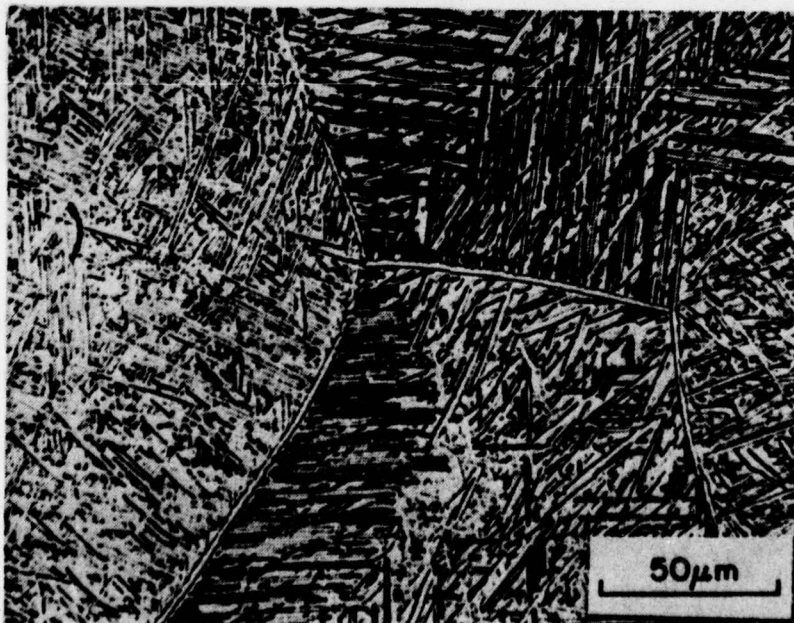
Figure 7. Specimen N5C (Figure 1). Note coarsening of grain boundary alpha.
