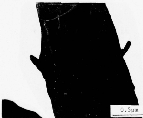
Figure 8. TEM of fiber extracted from as-grown composite showing side branches.
