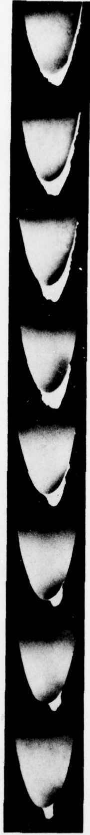
(a) 14 MINUTE HOVERING FLIGHT AT -14^{\circ}\text{C} AND L.W.C. 0.2\text{ g/m}^3 MAXIMUM ICE THICKNESS = 12.7 mm
