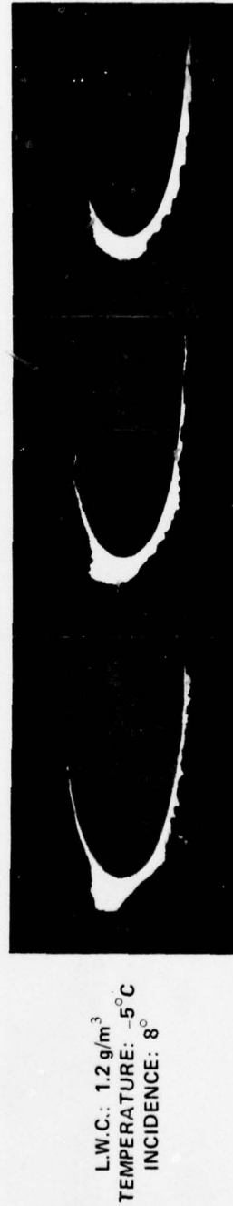
ICE ACCRETION PROFILES FROM WIND TUNNEL TESTS ON NACA 0015 AEROFOIL
