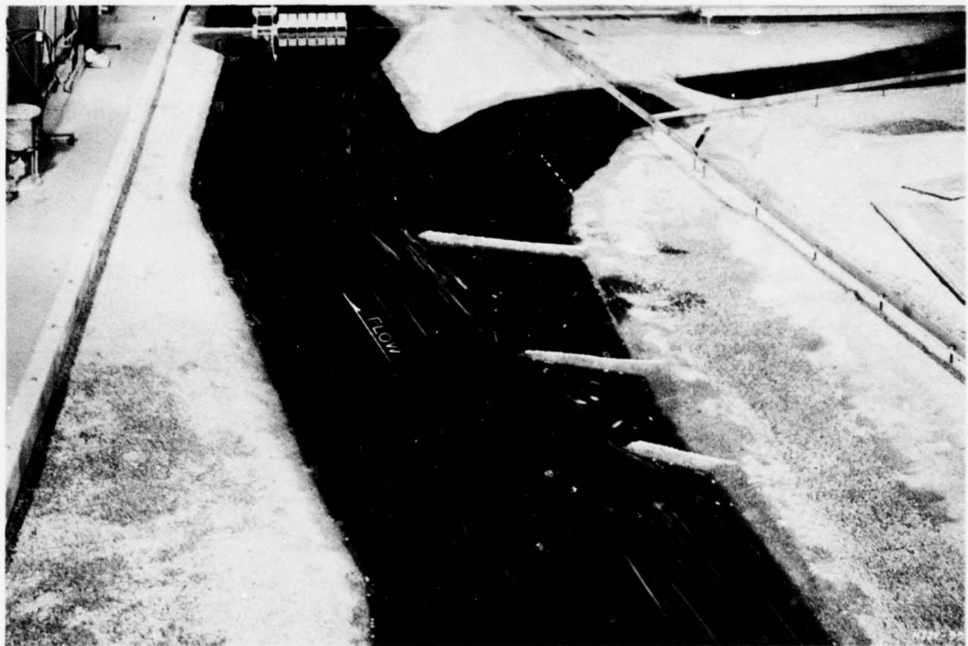
Photo 5. Plan D-modified; discharge 58,000 cfs, upper pool el 58.0. Surface current directions; note eddy in lock approach
