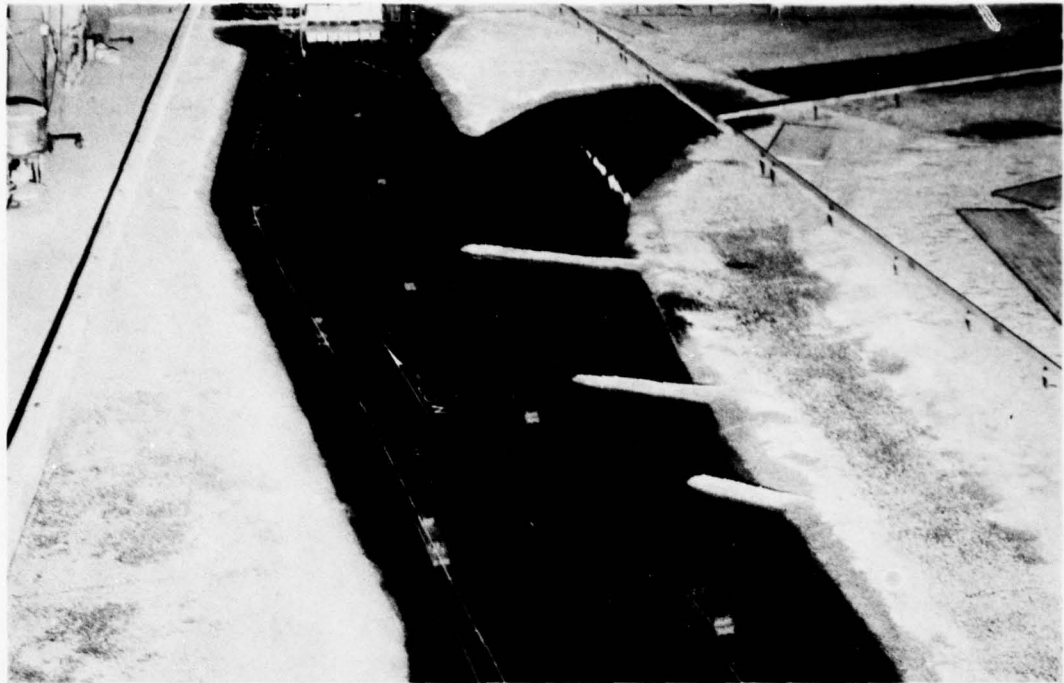
Photo 8. Plan D-modified; discharge 58,000 cfs, upper pool el 58.0. Paths of tows in upper lock approach. Downbound tow moving along left bank and upbound tow moving along right side
