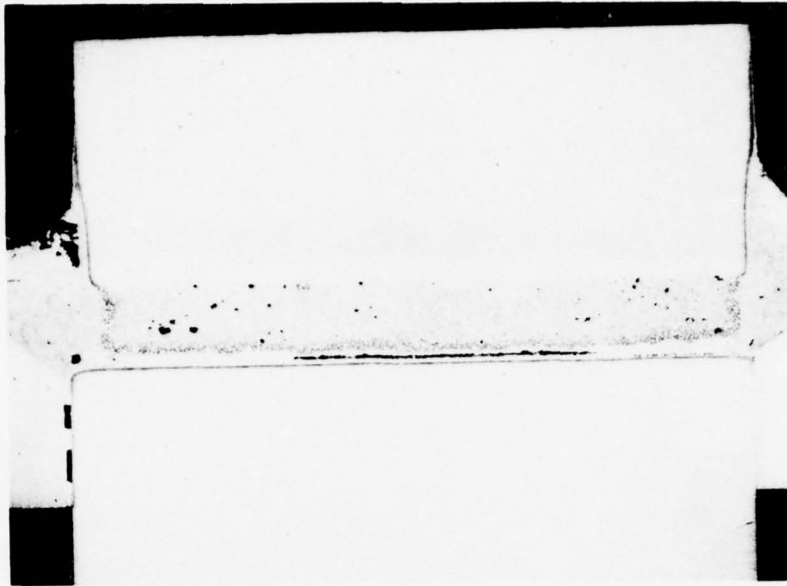
Figure 26. Braze Joint with S2 Sinter Filler Metal Which Had Cracked Before Brazing, 67 mil
