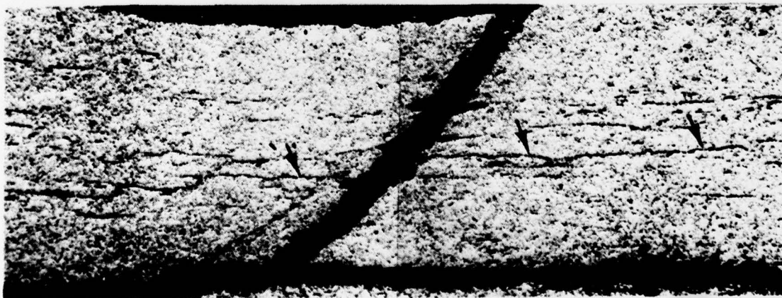
FIGURE 50. CROSS SECTION THROUGH TORN UPPER TUBE ILLUSTRATING THE 45° SHEAR, MECHANICAL FRACTURE APPEARANCE, TANK NO. 5.
