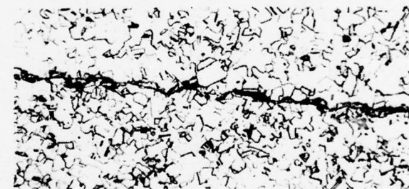
e) Area where melted material is almost continuous.
