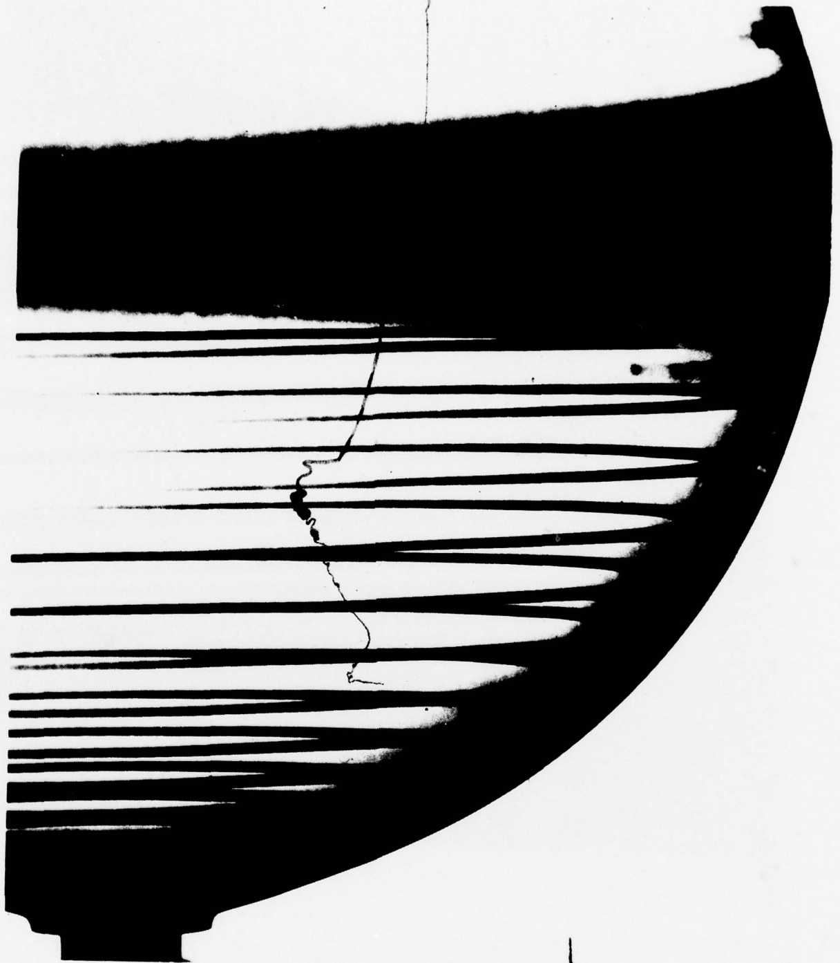
FIGURE 13. CONTACT PRINT OF RADIOGRAPH OF TANK NO. 4, AN ARDE RING STIFFENED DIAPHRAGM TANK, IN THE AS-RECEIVED CONDITION SHOWING COMPLETE EXPULSION.
