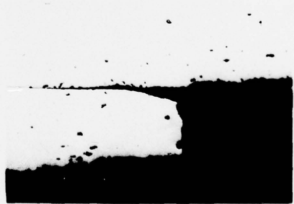
c) Section views showing slight attack in bond and along surface.
