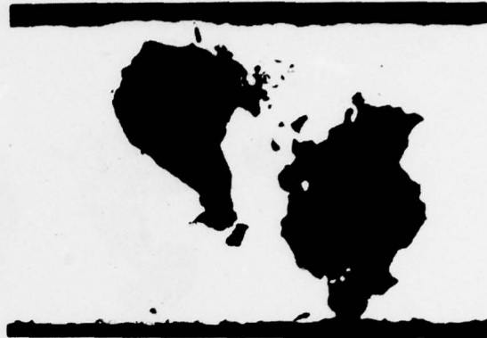
b) Section 0.0185 inch beyond initial site. Corrosion is approaching gas side surface for first time.
