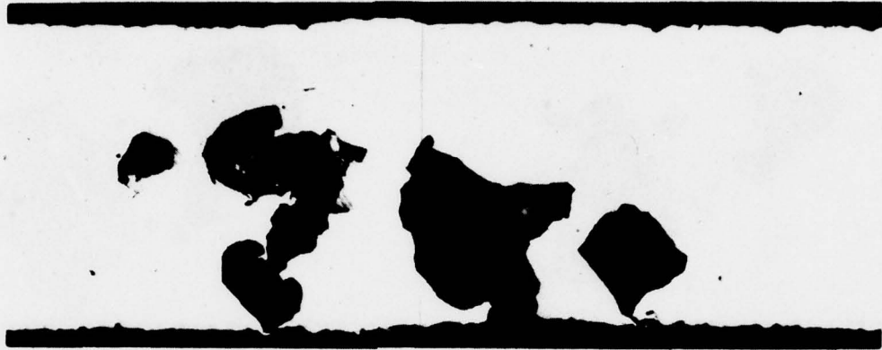
a) Section 0.007 inch beyond start of second pit, view (a) of Figure 36, and 0.025 inch beyond initial corrosion observation.
