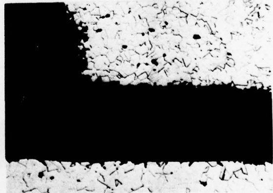
d) Cross section at start of crevice showing minor grain boundary attack.
