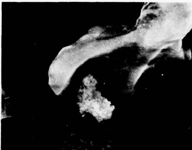
Figure 26. Agglomerate Smoke Particle Showing Botryoidal Structure (1800X Magnification)
