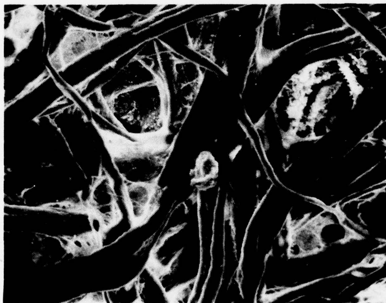
Figure 27. Smoke/Soot Particle on Filter Paper (600X Magnification)
