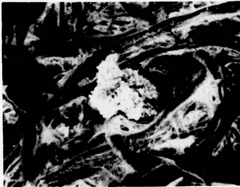
Figure 23. Compound Agglomerate Soot Particle (600X Magnification)
