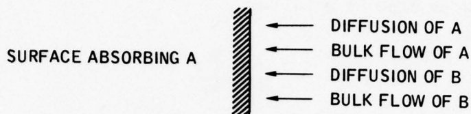
Figure 30. Diffusion Scheme for an Adsorbing Surface
