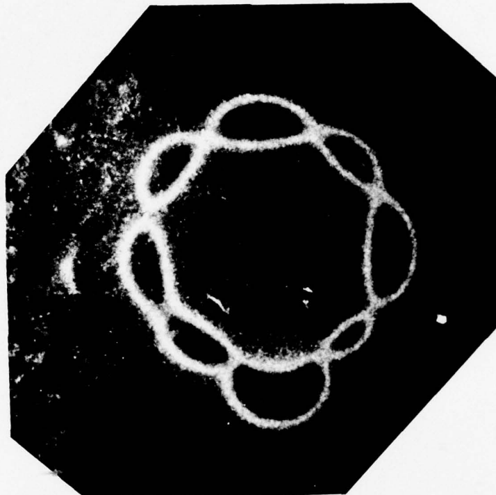
Figure 8. Liquid Crystal Display of Octagon Shaped Mode, Excited by Circumferential Loading
