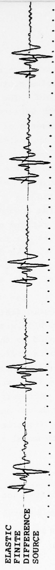
Figure 22. Short period seismograms from the elastic finite difference source are compared to the observations of the Pocatello Valley earthquake and the synthetic records from two analytical source models (Figure 8).
