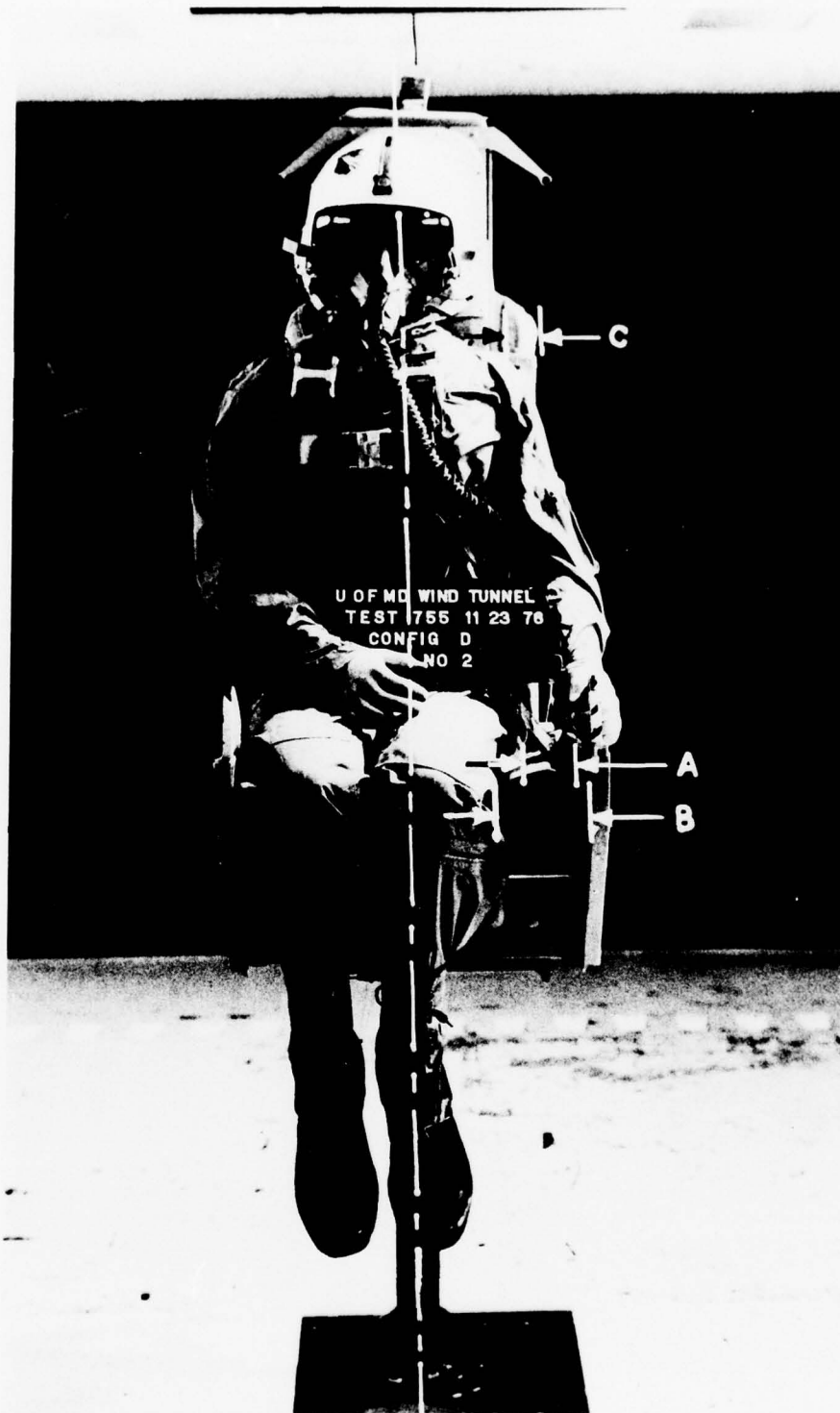
Figure 4. Anthropometric dummy in ACES II ejection seat. Configuration (D)
