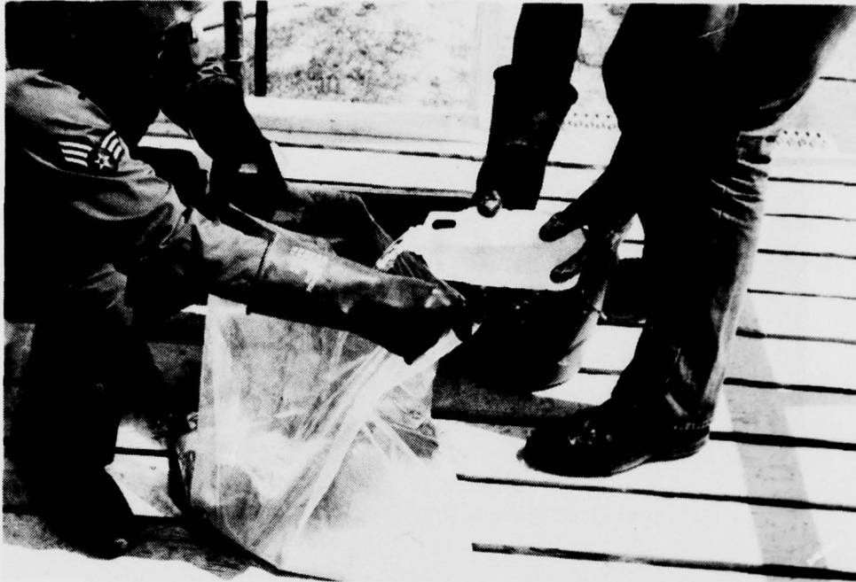
Figure 11 Adding One-Half Gallon of Liquid to the Powder
