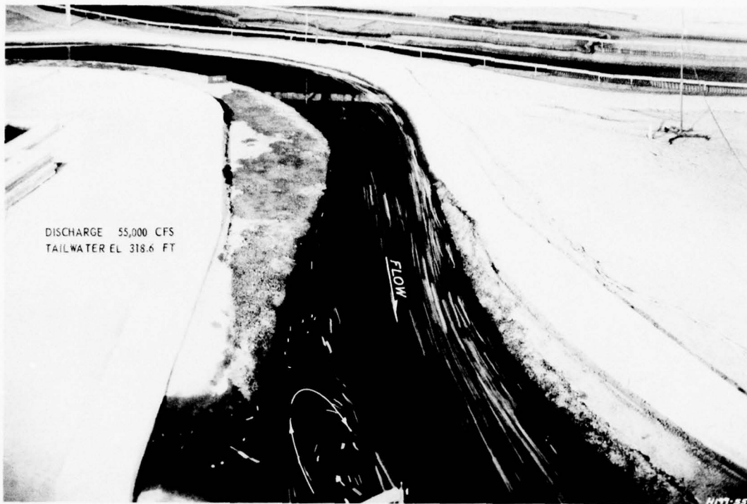
Photo 13. Plan C; surface currents approaching and through the bend at mile 25.6
