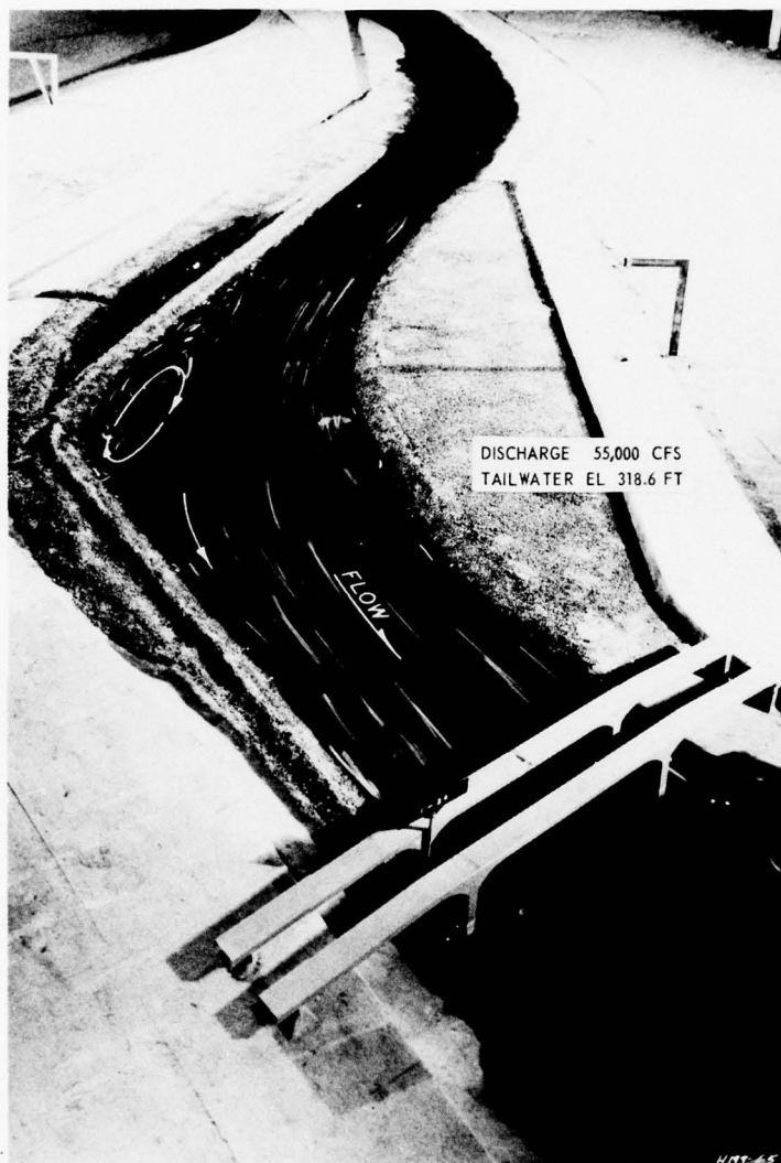
Photo 12. Plan C; surface currents through the bend at mile 28.1
