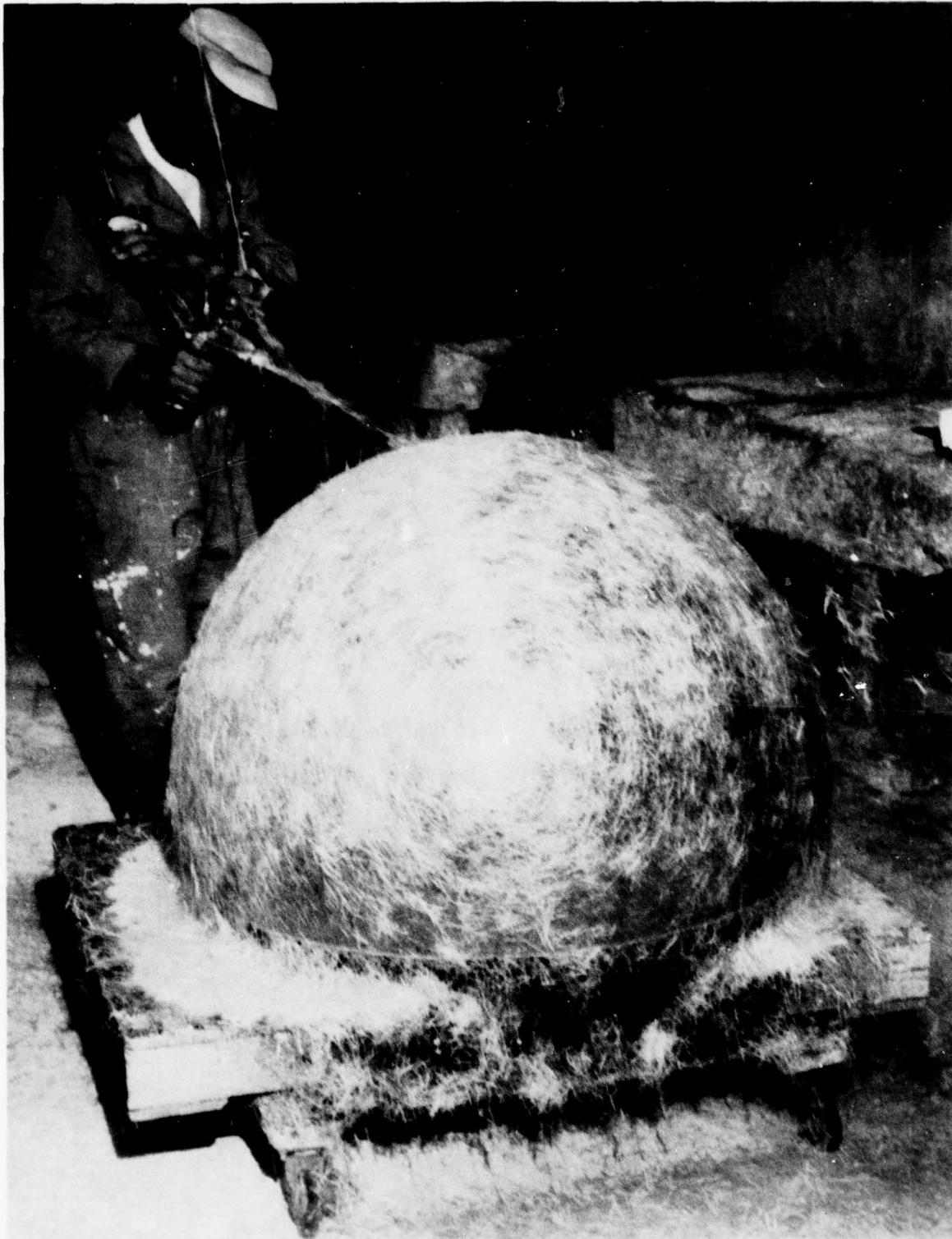
Figure 3-14. Application of Chopped Fiberglass to Aluminum Hemisphere
