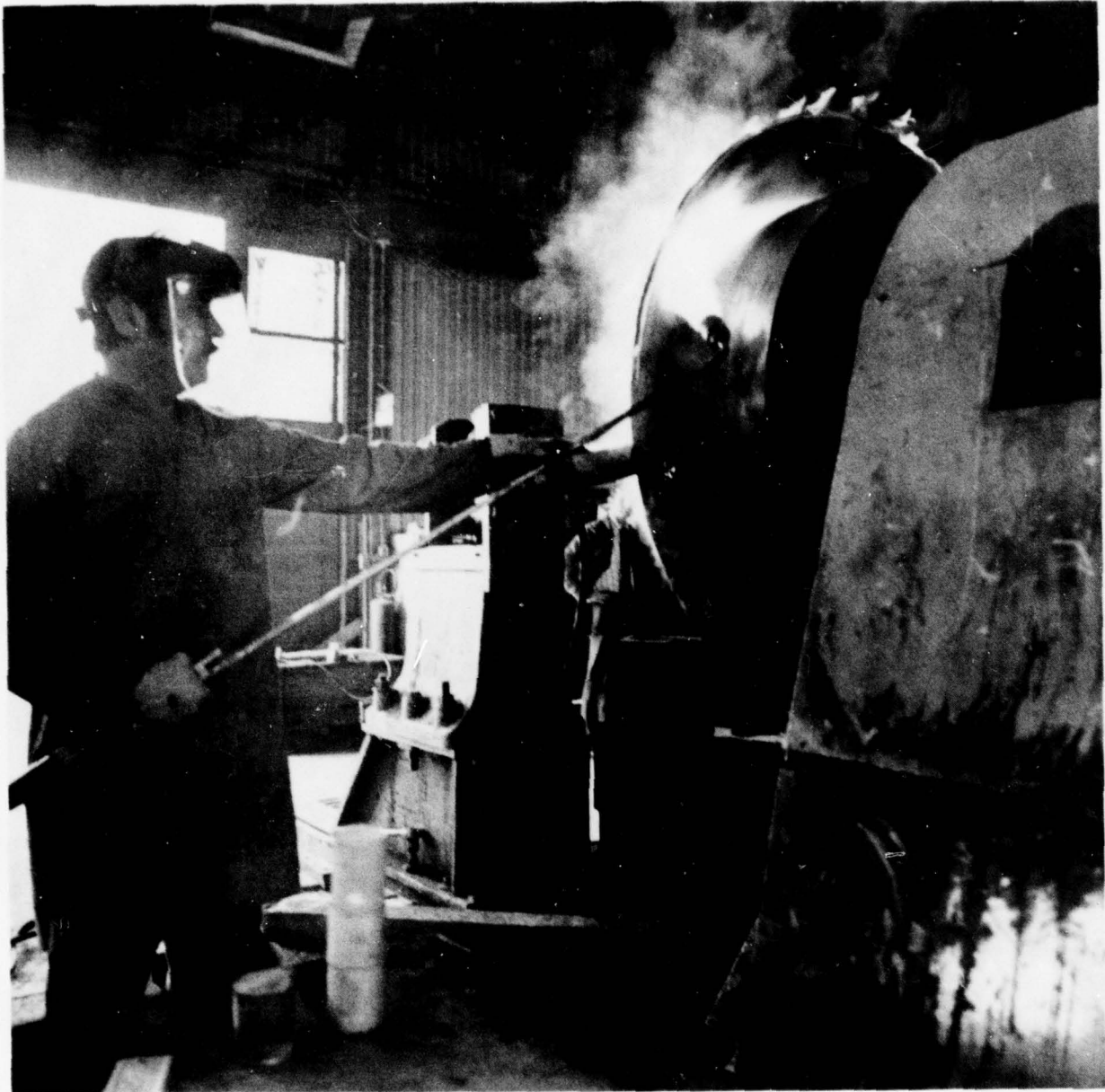
Figure 3-4. Spin Forming 60-Inch Diameter Aluminum Plate
