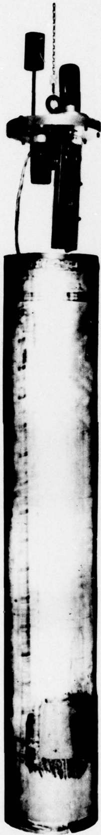
Fig. 1 Subsurface float with transistorized electronics pulled out for inspection. Float is 54 1/4 in. long and 8 5/8 in. o. d.
