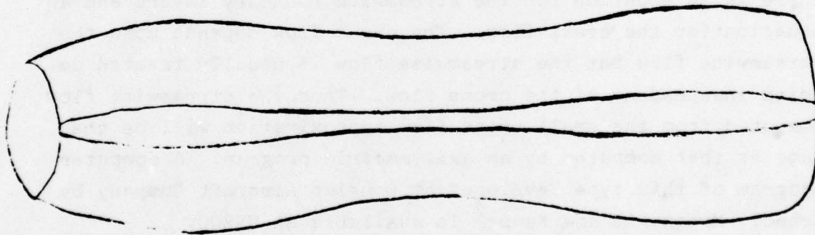
Figure 2 - Axisymmetric Pipe Model of a Three-dimensional Body for One Streamline
