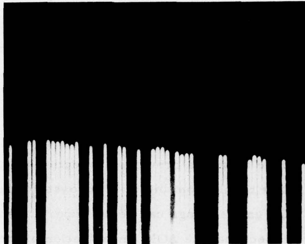
Figure 4.1.3.1-1. Spectral Analysis of AOM Output. TGA Gain = 5 Without AOM Linearization
