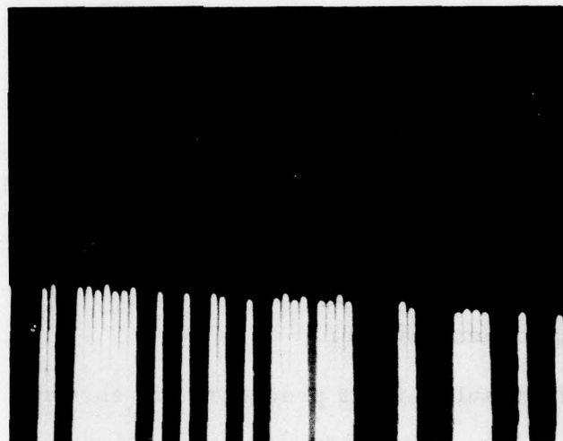
Figure 4.1.3.1-2. Spectral Analysis of AOM Output. TGA Gain = 5 With AOM Linearization
