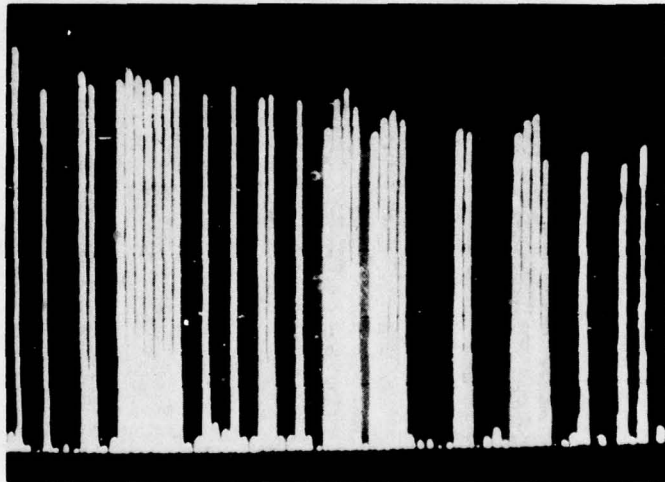
Figure 4.1.3.1-6. Spectral Analysis of AOM Output. TGA Gain = 11 With AOM Linearization
