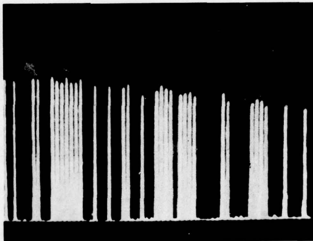
Figure 4.1.3.1-4. Spectral Analysis of AOM Output. TGA Gain = 8 With AOM Linearization
