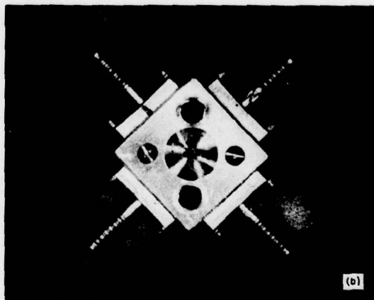
Fig. II-3. (a) Photograph of four GaInAsP/InP detectors mounted in (b) high-speed quad package.
