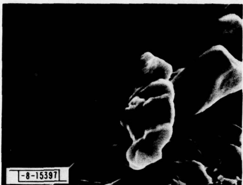
Fig.I-6. Scanning electron micrographs of output face of a DH laser which failed during operation at 50°C, apparently from a short circuit caused by indium extended from beneath device. As seen in lower view, indium makes contact with face.
