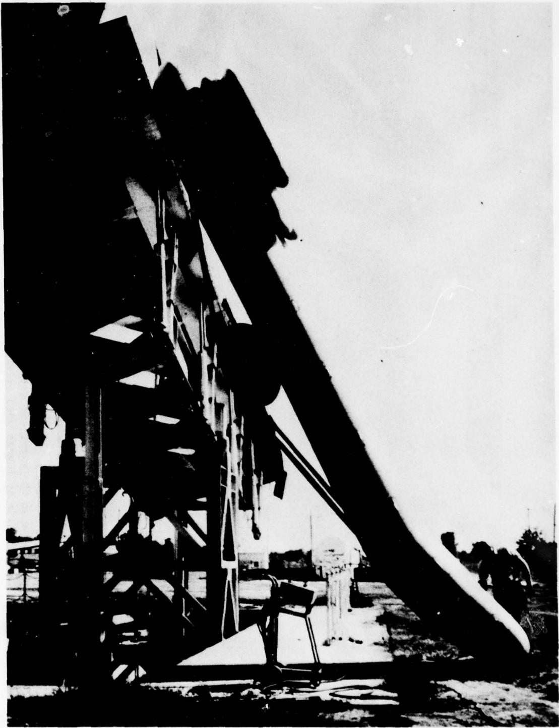
FIGURE 1. CAMI evacuation simulator showing slide deployed at a 68° angle.
