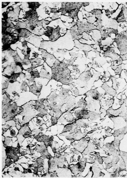
(b) GRAIN STRUCTURE AS VIEWED IN DEPOSITION DIRECTION
